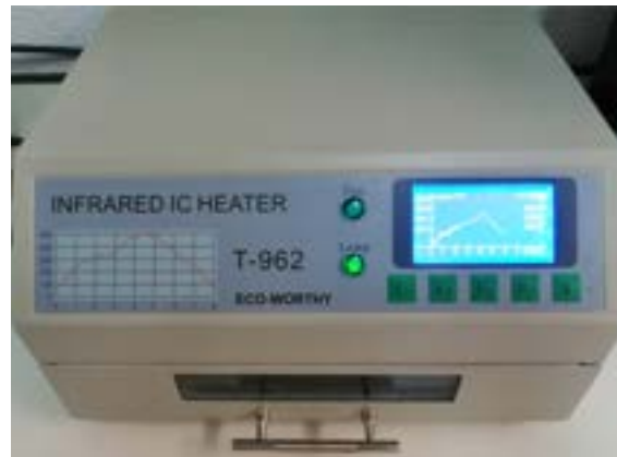
Figure 4.20: DCM's reflow oven with the time-temperature reflow profile used on screen.
