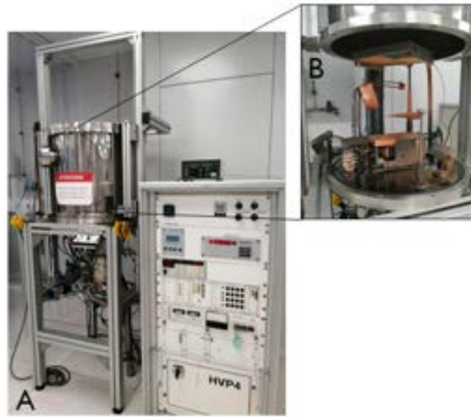
Figure 4.7: CEMOP's e-beam evaporation system. A - General view of the equipment. B - Detailed view of the equipment's interior.
