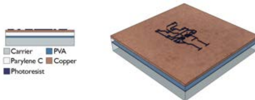
Figure 4.11: Patterned photoresist succeeding the development step. The pattern corresponds to one of the electrical circuits from the light emitting diode (LED) prototype.
