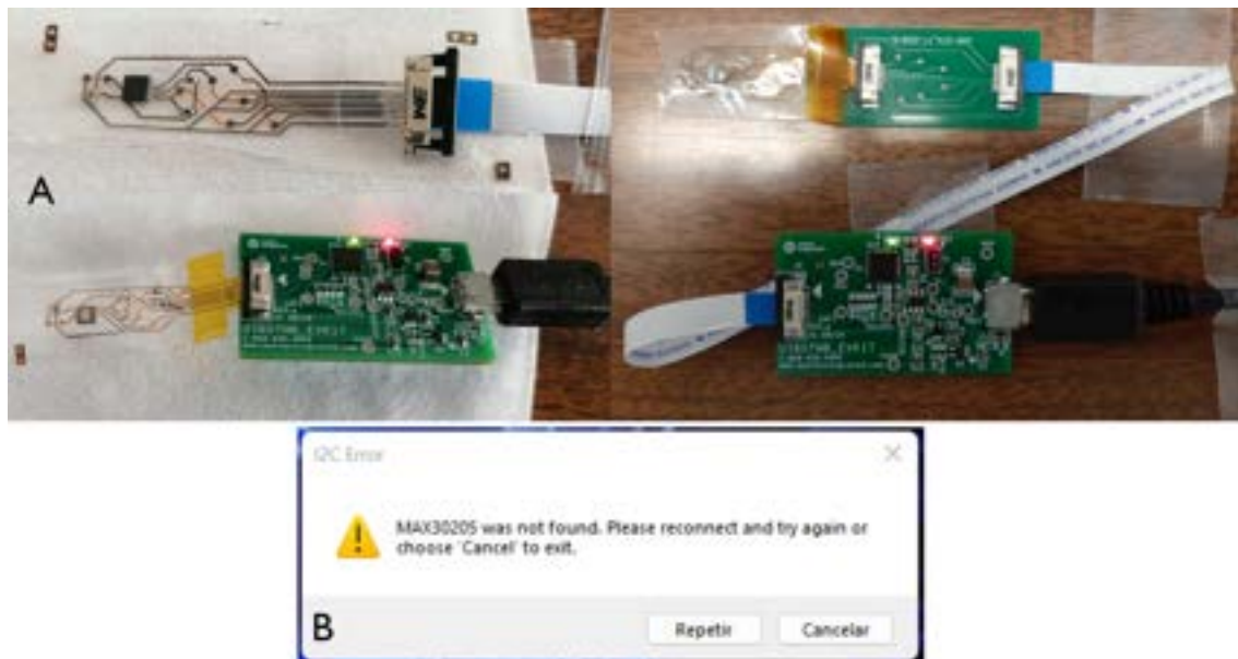
Figure 5.23: Tests performed to the MAXIM prototype (A) and the warning message displayed in Maxim Evaluation kit's program succeeding each test (B).
