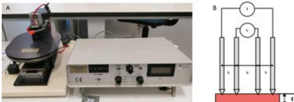
Figure 4.28: Representation of the four-point-probe method. A - CENIMAT's Jandel 4-Point Probe System. B - 4-Point Probe operation principles.
