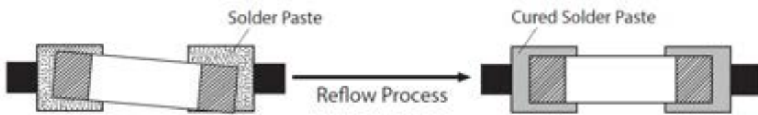
Figure 3.4: Self-alignment of rigid silicon components after the reflow process, from [8].
