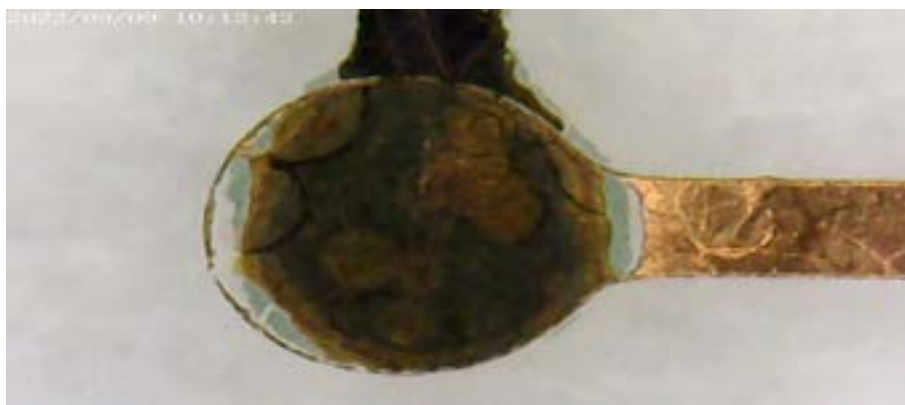
Figure 5.9: Unwanted metal removal due to the over-etching of the copper layer.
