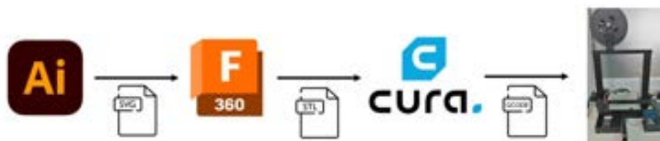
Figure 4.25: Steps involved in the production the 3D carrier support.
