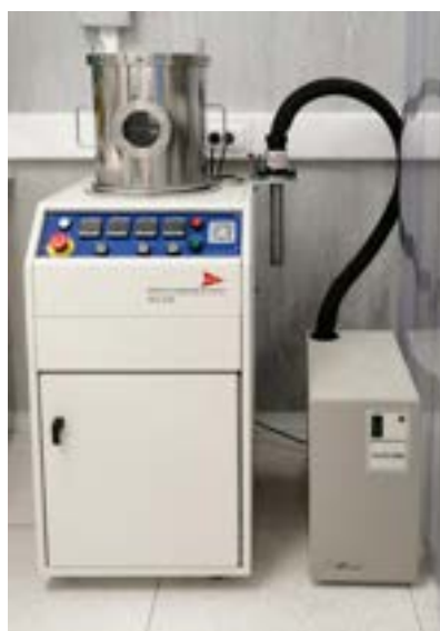
Figure 4.5: CVD system responsible for the deposition of parylene.
