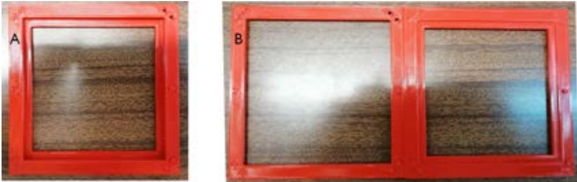
Figure 5.4: Final result of the carrier support manufactured via laser technology. A - Exhibits an assemble carrier support. B - Shows the disassembled state of the support.
