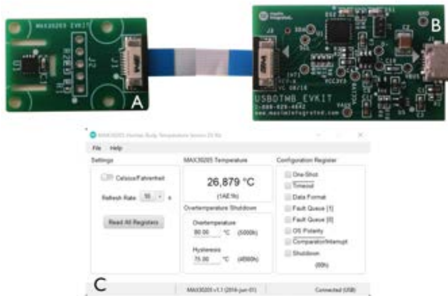
Figure 2.9: MAX30205 Human Body Temperature Sensor Evaluation Kit. A - Temperature Sensor PCB with the MAX30205 human body temperature sensor. B - USBDTMB PCB, which controls the communication of the raw temperature data to the computer. C - GUI program supplied by Maxim Integrated.
