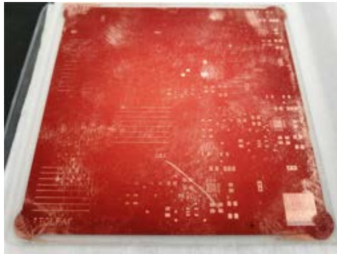
Figure 5.6: PT100's electrical circuit etched onto the copper layer.
