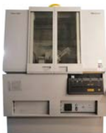
Figure 4.29: CENIMAT's X'Pert PRO MRD system responsible for the XRD method.
