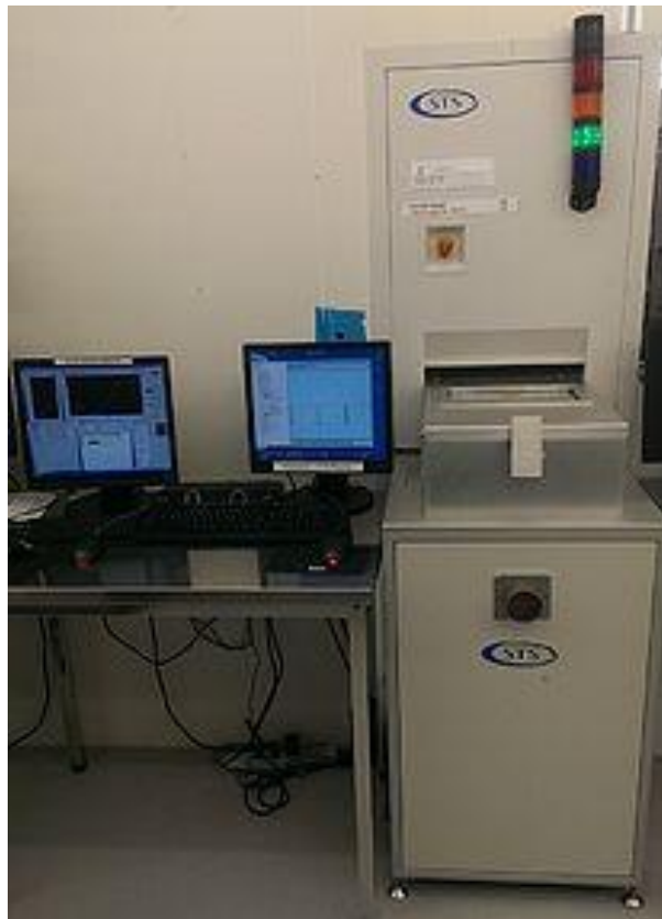
Figure S4 – Image of the ICP etch tool, primarily dedicated to etching III-V materials, used in this study. III-V PRO ICP, serial number MP0647, from SPTS. The picture was obtained from a closed-access DTU database.
