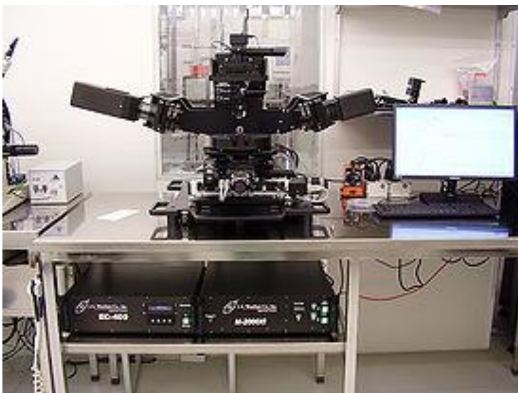
Figure S6 - Image of the VASE ellipsometer tool used to characterize the samples in the ‘Oxidation Study’. M2000XI-210 ellipsometer from J.A. Woollam Co., Inc.. The picture was obtained from a closed-access DTU database.
