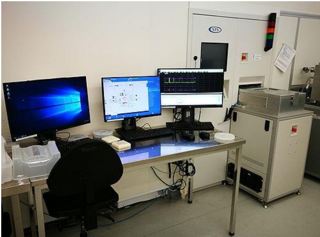
Figure S3 – Image of the DRIE tool used in this work. Nemotek Advanced DRIE Pegasus 2, serial number MP0641, from SPTS. The picture was obtained from a closed-access DTU database.
