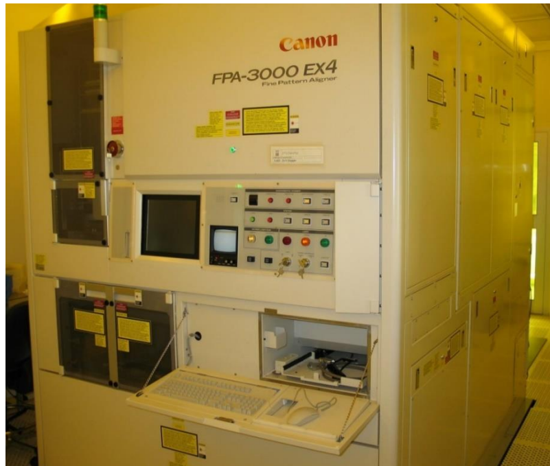
Figure S. 3- DUV Stepper from Canon (FPA-3000EX4 Stepper system), with excimer laser unit 248 nm wavelength. Picture adapted from a closed-access DTU database.
