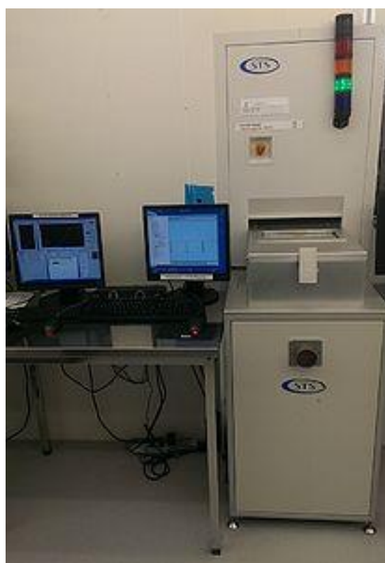
Figure S. 5- III-V ICP tool, Inductively Coupled Plasma, SPTS serial number MP0647. Picture adapted from a closed-access DTU database.
