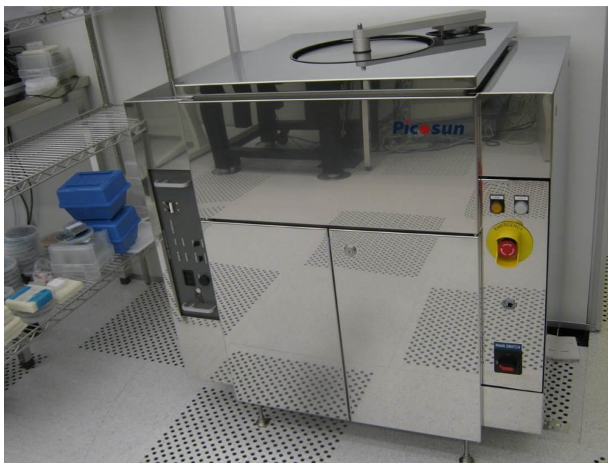
Figure S. 4- Picosun thermal atomic layer deposition model R200 equipment. The tool is able to deposit a very thin layer of \text{Al}_2\text{O}_3 , \text{TiO}_2 (amorphous or anatase), \text{HfO}_2 , \text{ZnO} and AZO (Al-doped \text{ZnO} ) on different samples. Picture adapted from a closed-access DTU database.
