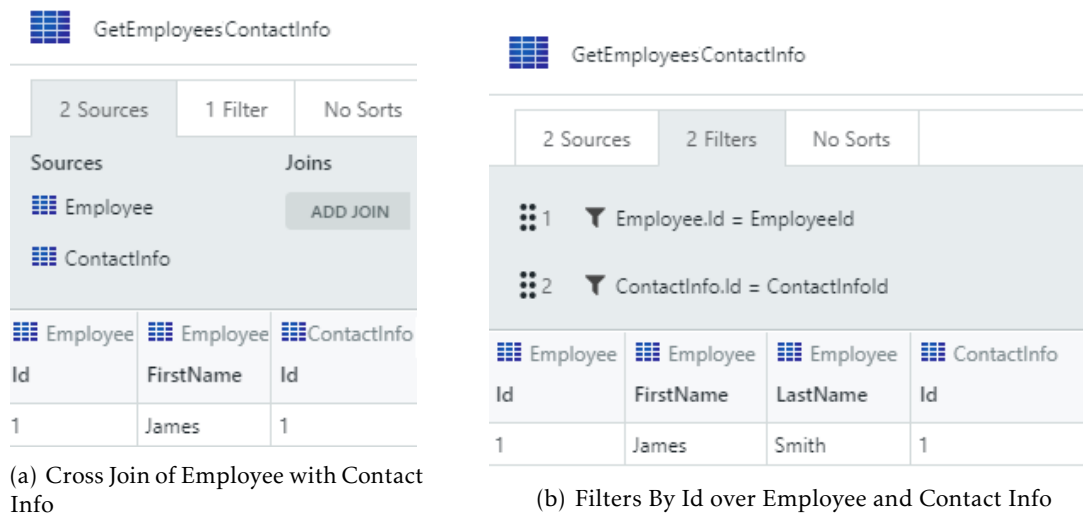
Figure 7.9: Cross Join of two Sources with two Filters By Id Example in OutSystems
