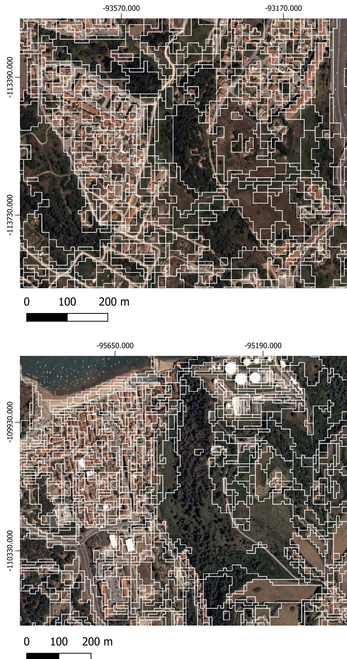
Figure 7.4: Example areas of segmentation J . Urban areas are finely segmented, whereas natural areas have less precise separation and non-homogeneous segments.
