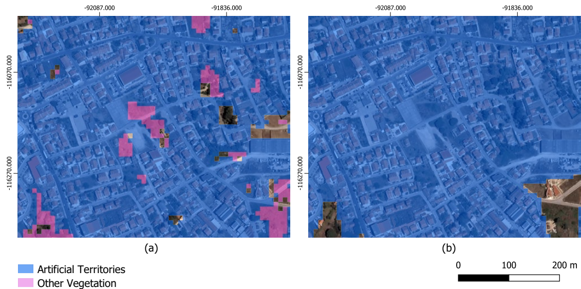
Figure 6.9: Classification examples of PBIA_map (a) and COS (b) with orthophoto background. PBIA_map identifies small areas of vegetation, not represented in COS .
