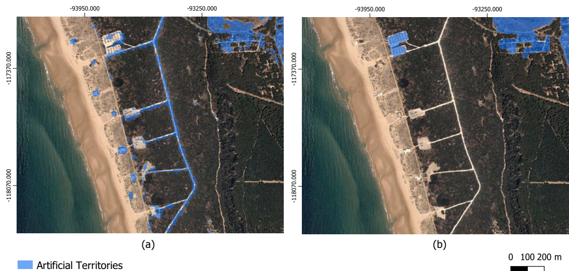
Figure 6.5: Classification examples of PBIA_map (a) and COS (b) with orthophoto background. PBIA_map is able to classify small roads and buildings, not represented in COS .
