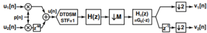
Figura 2.17 - Modulador Sigma-Delta de 2 canais com filtro \pi -shifted. Fonte: R. S. A. Kumar and N. Krishnapura, "A 2-Channel ADC Using a Delta-Sigma Modulator Without Reset & a Modulated-Sinc-Sum Filter," ESSCIRC 2019 - IEEE 45th Eur. Solid State Circuits Conf. , pp. 365–368, 2019, doi: 10.1109/ESSCIRC.2019.8902610.
