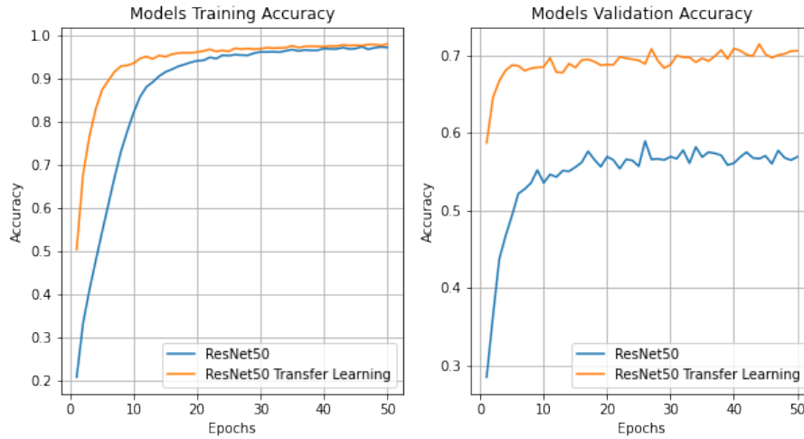
Figure 5.2: Comparison of the accuracy values between ResNet50 with and without Transfer Learning Technique
