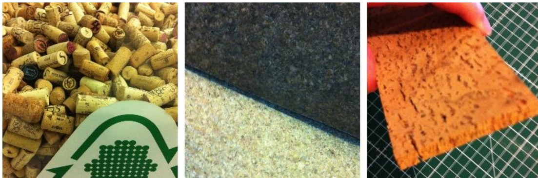
Figure 102. From left to right, recycled cork, agglomerated cork sheets, natural cork stripes
