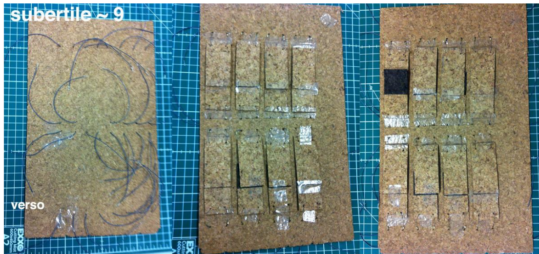
Figure 109. Subtile testing, pixels and S.M.A. wire assembly, square and rectangular shape pixels
