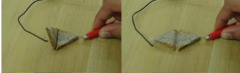
Figure 19. Hybrid: Playing with cork and flexinol
