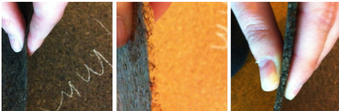
Figure 103. Dark and light agglomerated cork, 1, 2, 3 mm cuts, sponsored by Amorim
