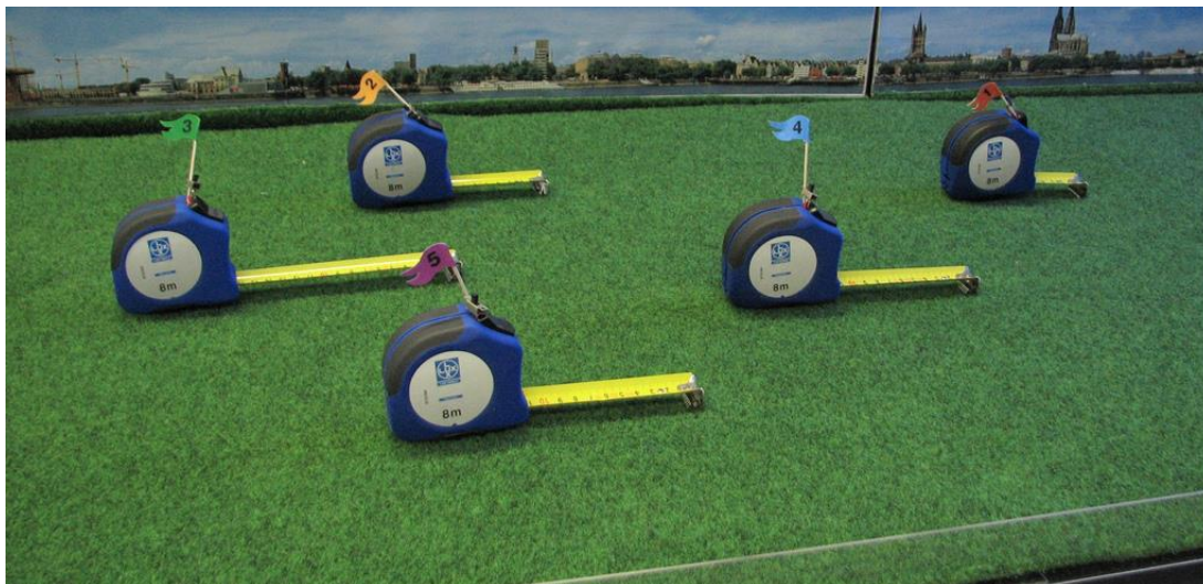
Figure 53. Meter crawler by Keiko Takahashi, 2013, retrieved from https://makezine.com/2010/11/16/meter-crawler-a-robot-made-from-a-t/
