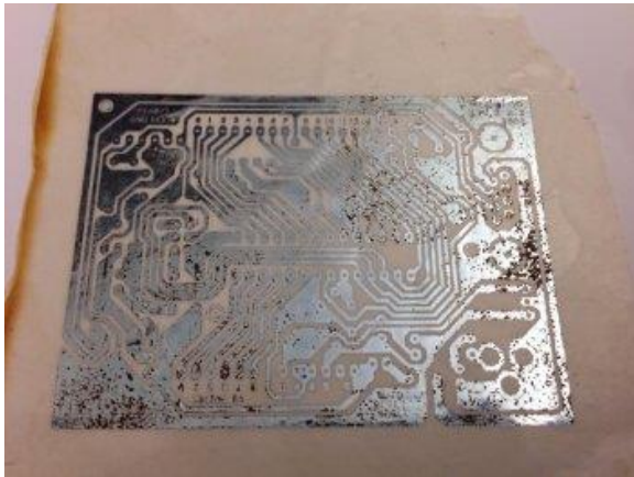
Figure 129. Biodegradable circuit printed onto material made of cellulose acetate, by Lynn Rothschild, retrieved from http://2014.igem.org/Team:StanfordBrownSpelman/Building_The_Drone
