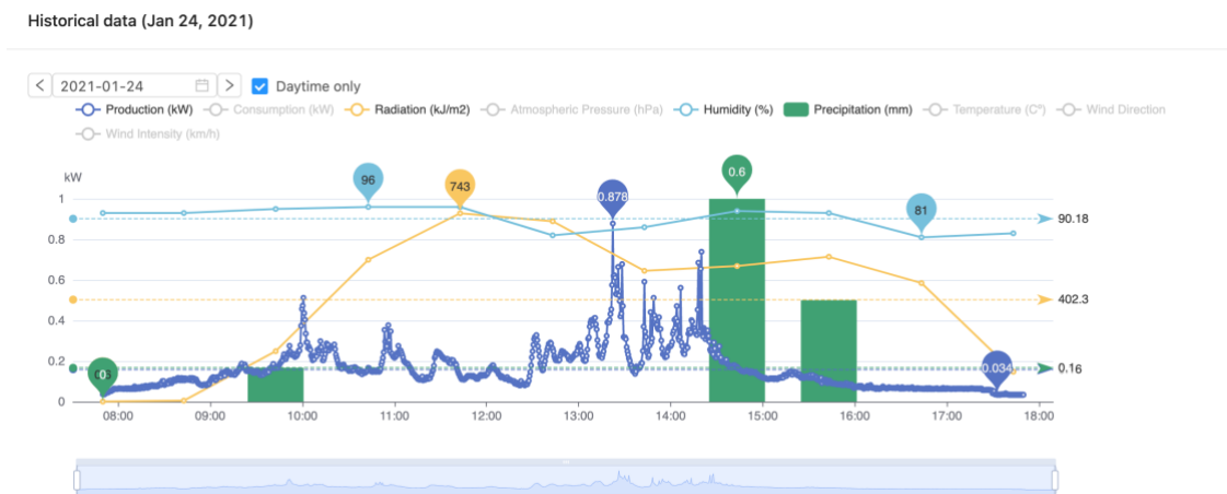
Figure 4 – Readings on 2021-01-24 of energy production, radiation, humidity and precipitation
