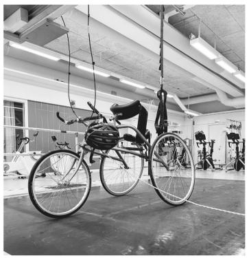
Picture of setup for Frame Running incremental treadmill test (FRITT) at Bosön National Sports Confederation's laboratory for performance in Stockholm
