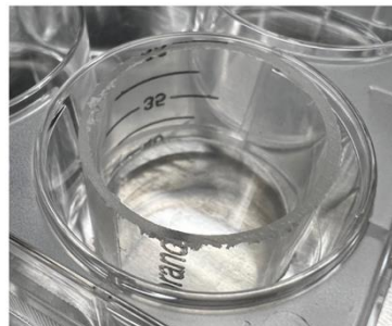
Figure 10. Falcon tube cut to a height of 18 cm to push the mesh to the bottom of the 6-well plate.
