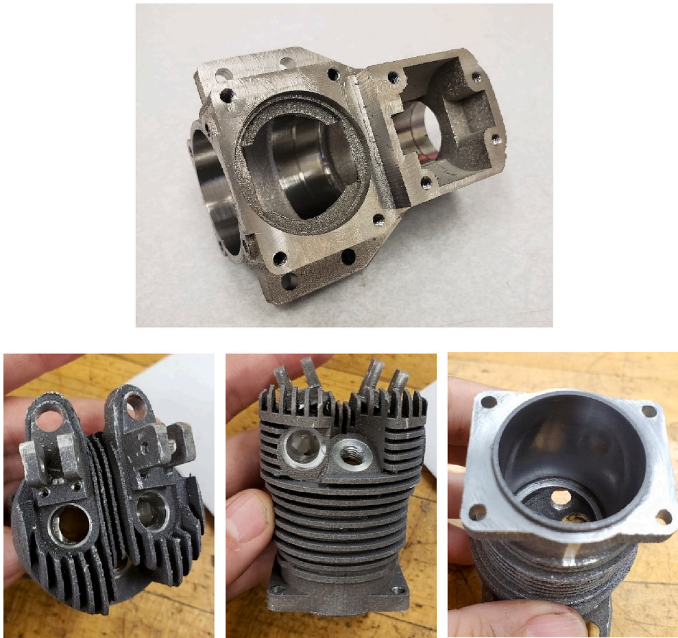
Fig. 13. Finished AM crankcase (top) and cylinder head (bottom).
