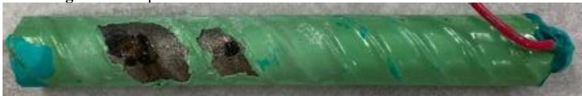
Figure 3.21: Specimen ECR2-UV-100-4 anode bar after disbondment test
