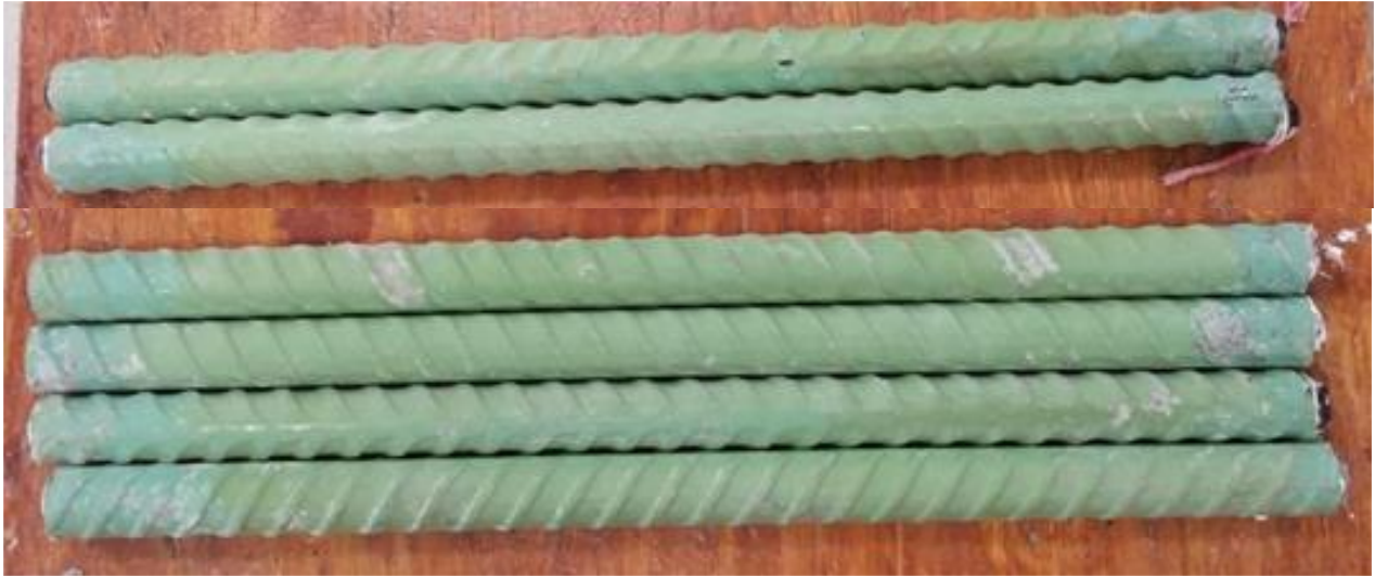
Figure 3.68: Top bars (top) and bottom bars (bottom) of specimen SE-ECR1-UV-1000-ND-1 after 96 weeks of testing
