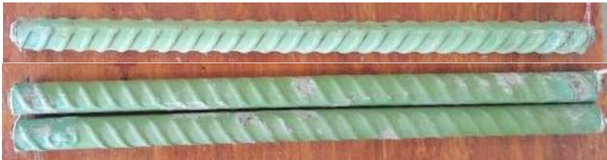
Figure 3.71: Top bar (top) and bottom bars (bottom) of specimen CB-ECR1-UV-1000-ND-1 after 96 weeks of testing
