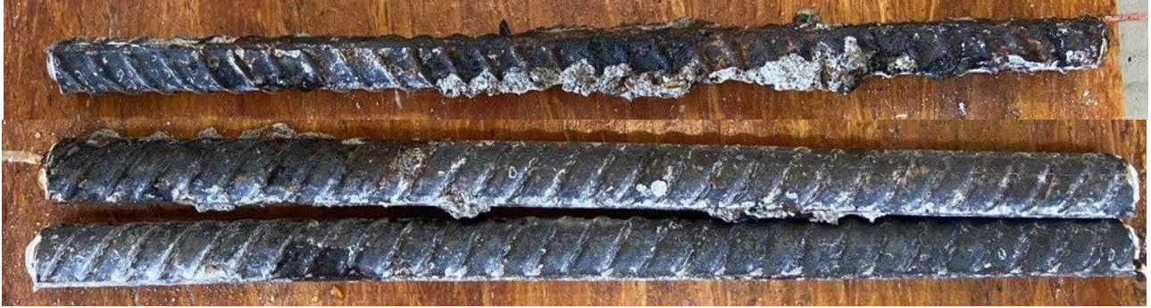
Figure 3.85: Top bar (top) and bottom bars (bottom) of specimen CB-Conv-B-IPANEX-1 after 96 weeks of testing
