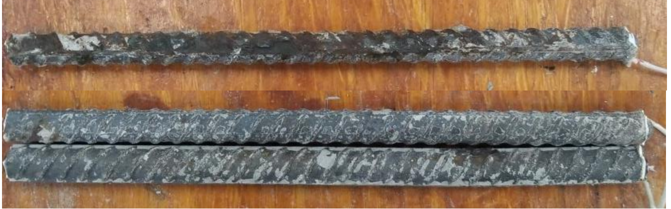
Figure 3.87: Top bar (top) and bottom bars (bottom) of specimen CB-Conv-B-Xypex-2 after 96 weeks of testing
