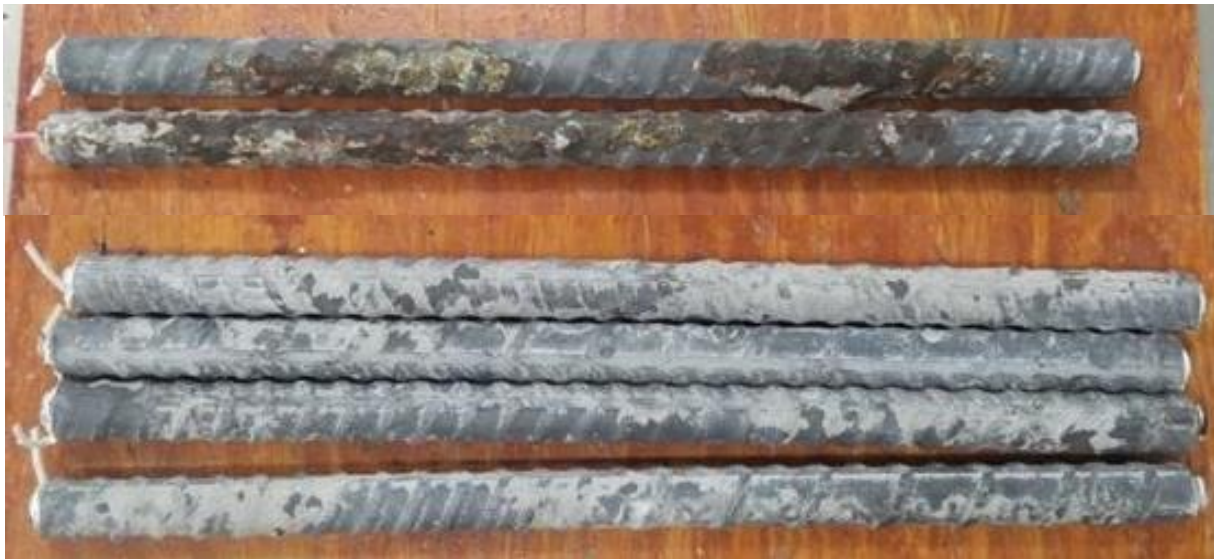
Figure 3.78: Top bars (top) and bottom bars (bottom) of specimen SE-ChromX-5 after 96 weeks of testing
