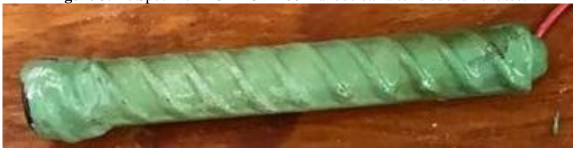
Figure 3.22: Specimen ECR-UV-1000-ND-6 anode bar after 15 weeks of rapid macrocell testing
