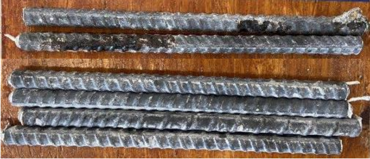
Figure 3.79: Top bars (top) and bottom bars (bottom) of specimen SE-ChromX-IPANEX-2 after 96 weeks of testing
