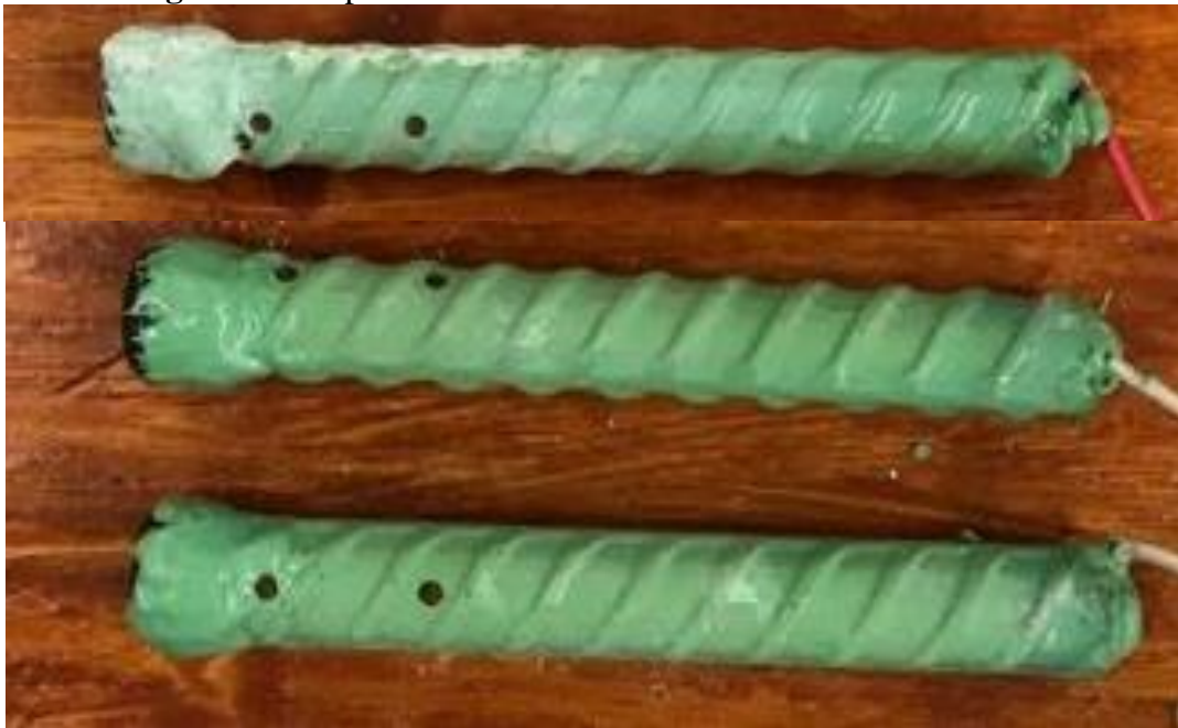
Figure 3.17: Specimen ECR1-UV-1000-4 anode bar (top) and cathode bars (bottom) after 15 weeks of rapid macrocell testing
