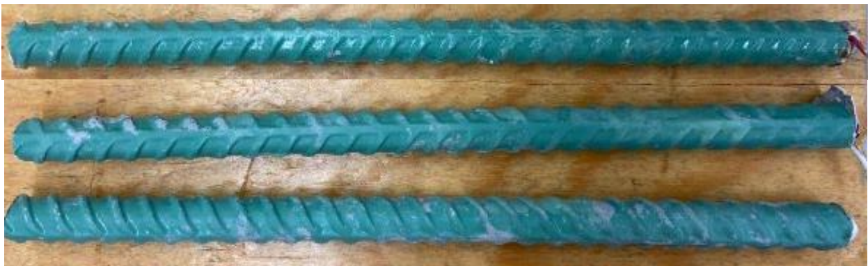
Figure 3.64: Top bars (top) and bottom bars (bottom) of specimen CB-ECR1-ND-2 after 96 weeks of testing
