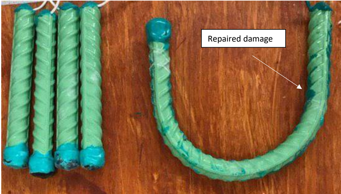
Figure 3.15: Specimen ECR1-5 anode bar (right) and cathode bars (left) after 15 weeks of rapid macrocell testing
