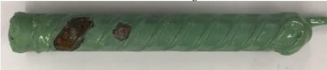
Figure 3.16: Specimen ECR1-2 anode bar after disbondment test
