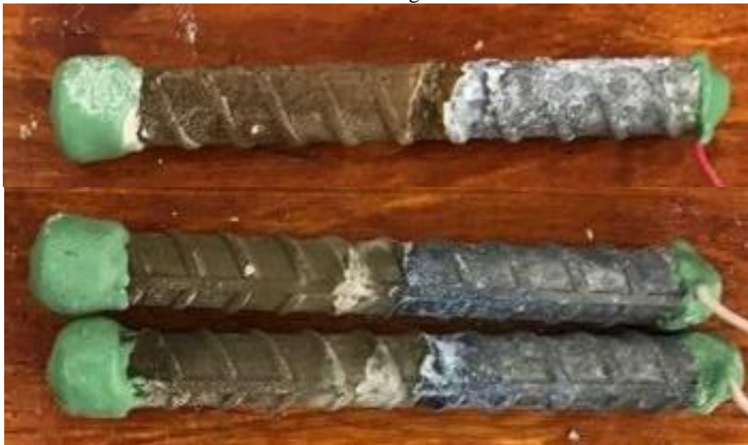
Figure 2.5: Specimen A1094-4 anode bar (top) and cathode bars (bottom) after 15 weeks of rapid macrocell testing
