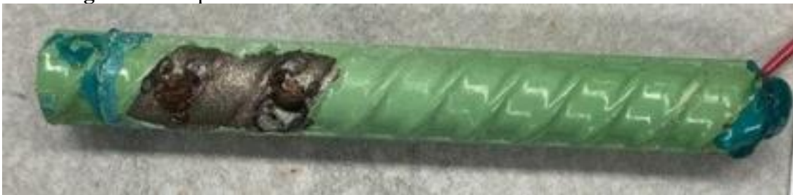
Figure 3.20: Specimen ECR2-UV-200-3 anode bar after disbondment test
