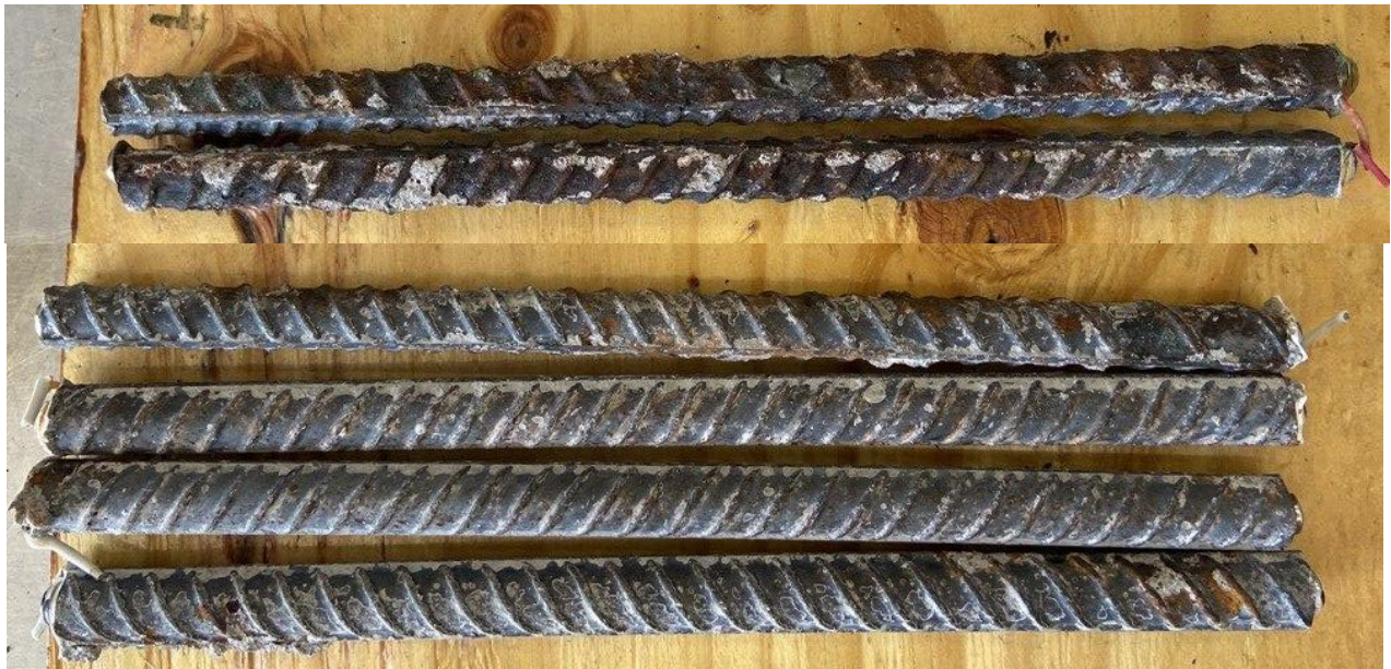
Figure 3.84: Top bar (top) and bottom bars (bottom) of specimen SE-Conv-B-IPANEX-2 after 96 weeks of testing
