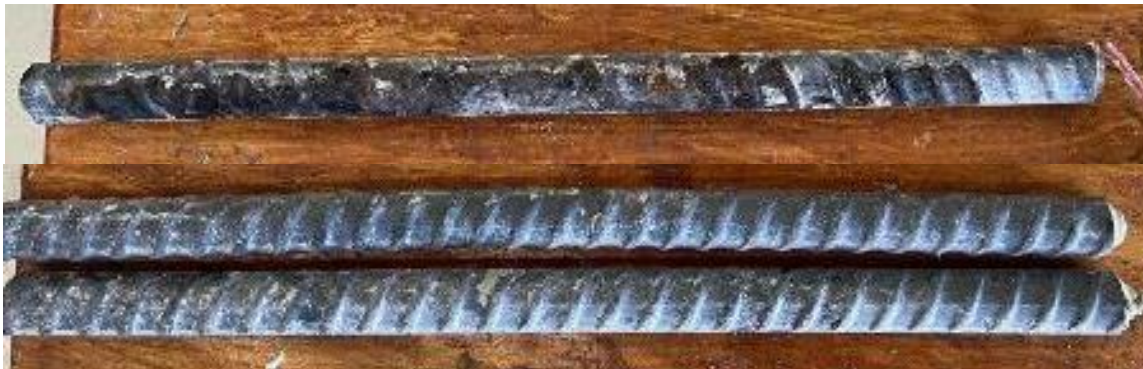
Figure 3.57: Top bar (top) and bottom bars (bottom) of specimen CB-Conv-B-4 after 96 weeks of testing
