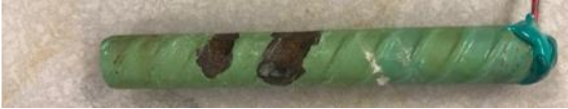
Figure 3.18: Specimen ECR1-UV-1000-4 anode after disbondment test
