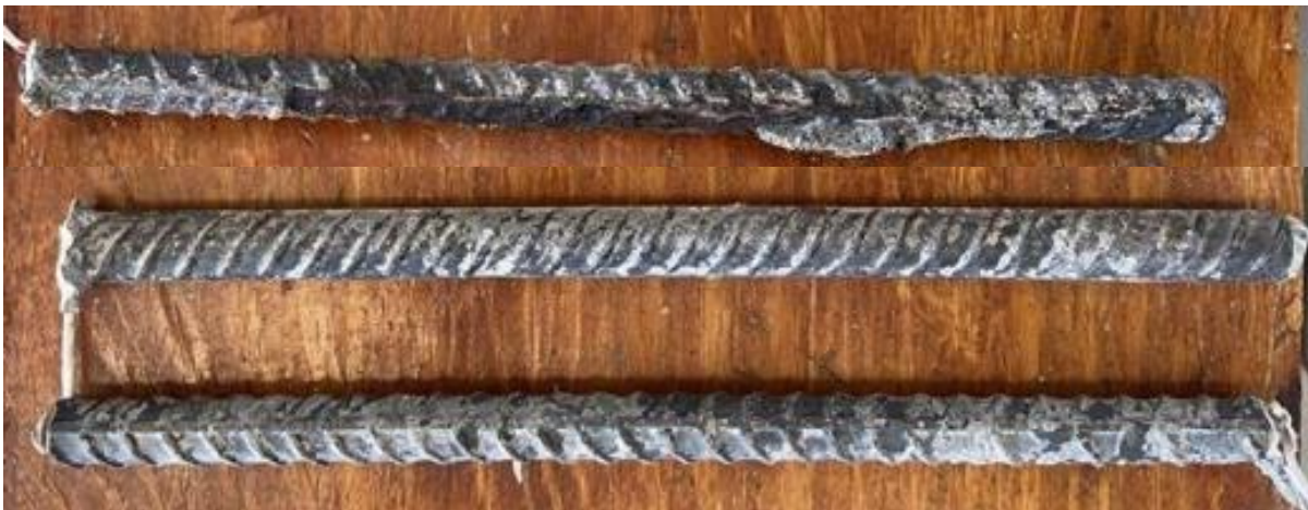
Figure 3.83: Top bar (top) and bottom bars (bottom) of specimen CB-ChromX-Xypex-2 after 96 weeks of testing
