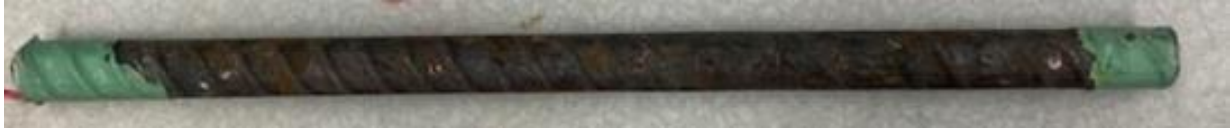
Figure 3.70: Top bar of specimen CB-ECR1-UV-1000-2 after disbondment test
