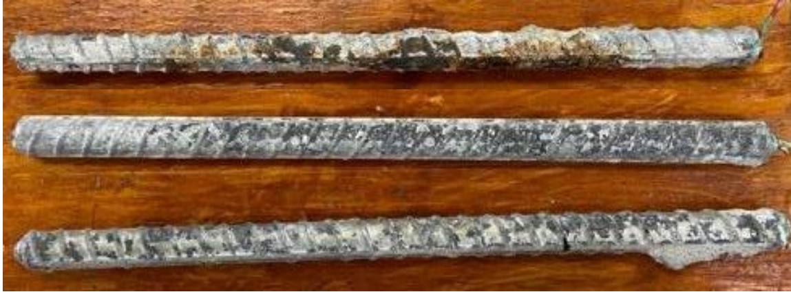
Figure 3.75: Top bar (top) and bottom bars (bottom) of specimen CB-A1094-6 after 96 weeks of testing
