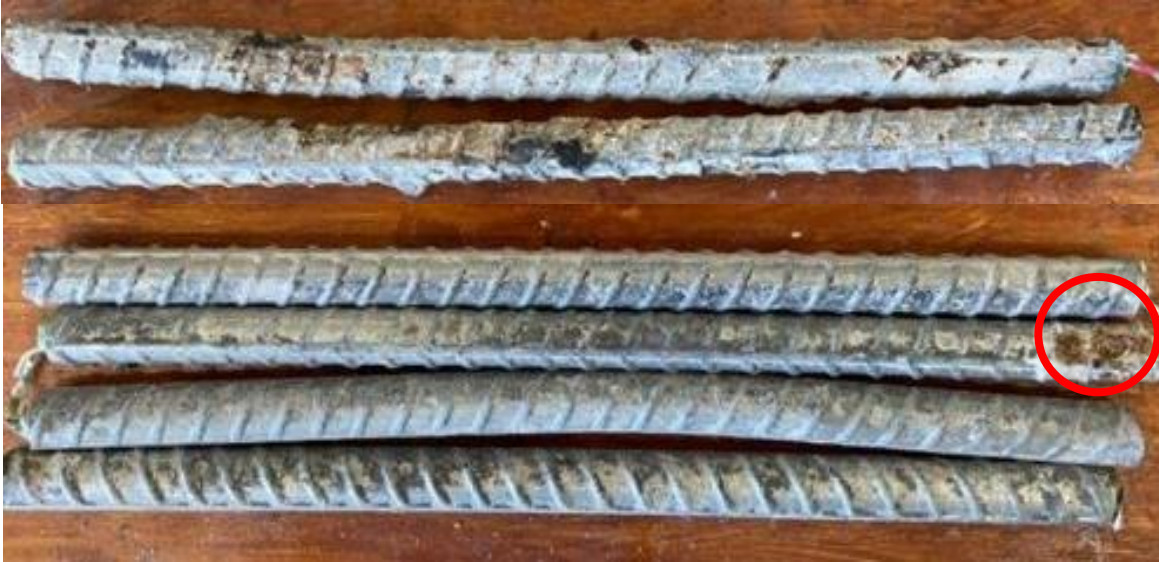
Figure 3.72: Top bars (top) and bottom bars (bottom) of specimen SE-A767-2 after 96 weeks of testing
