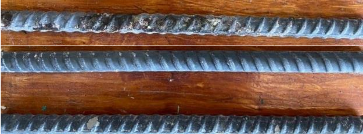
Figure 3.81: Top bar (top) and bottom bars (bottom) of specimen CB-ChromX-1 after 96 weeks of testing
