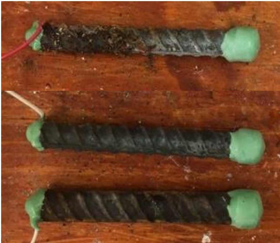
Figure 3.13: Specimen Conv-B-5 anode bar (top) and cathode bars (bottom) after 15 weeks of rapid macrocell testing
