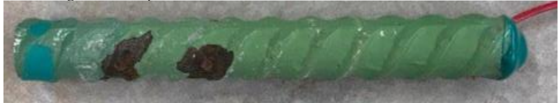
Figure 3.19: Specimen ECR1-UV-500-5 anode bar after disbondment test
