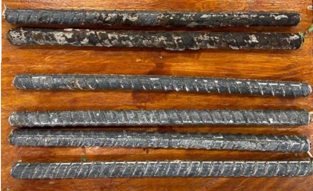
Figure 3.55: Top bars (top) and bottom bars (bottom) of specimen SE-Conv-C-1 after 96 weeks of testing
