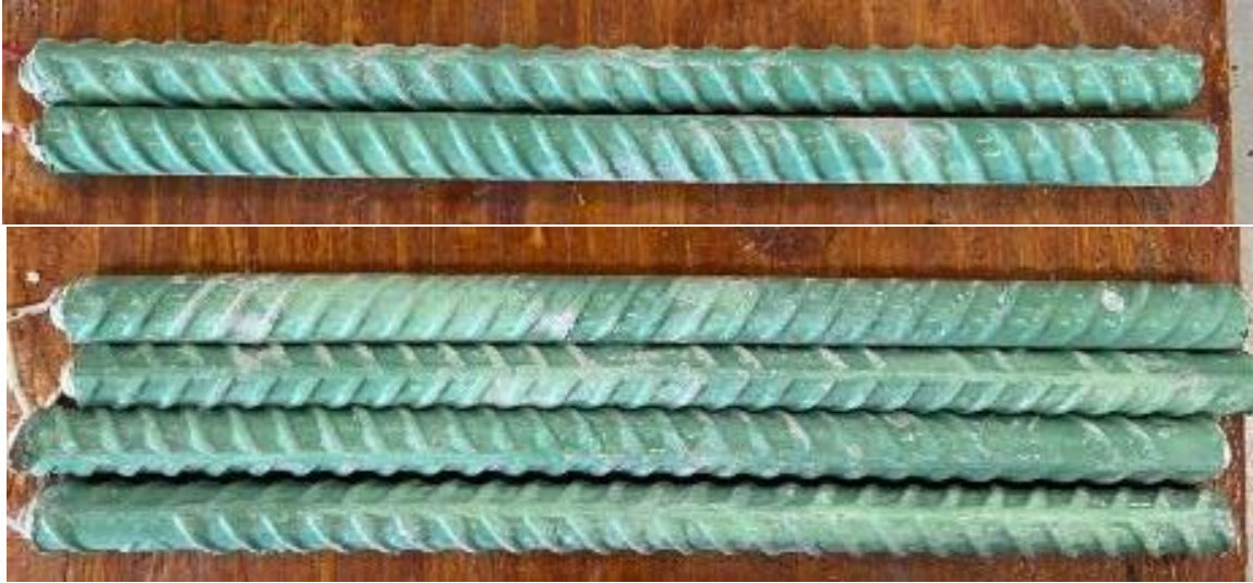
Figure 3.61: Top bars (top) and bottom bars (bottom) of specimen SE-ECR1-ND-2 after 96 weeks of testing
