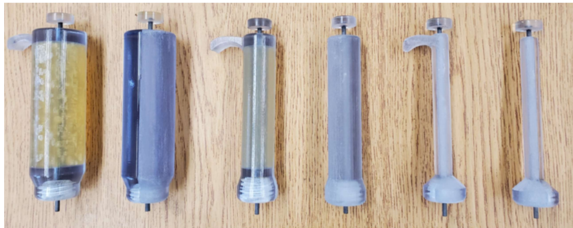
Figure 5.2. Micropipette handles with varying diameter and finger rest presence. From left to right: 40 mm diameter with and without a finger rest, 25 mm diameter with and without a finger rest, 12 mm diameter with and without a finger rest.
