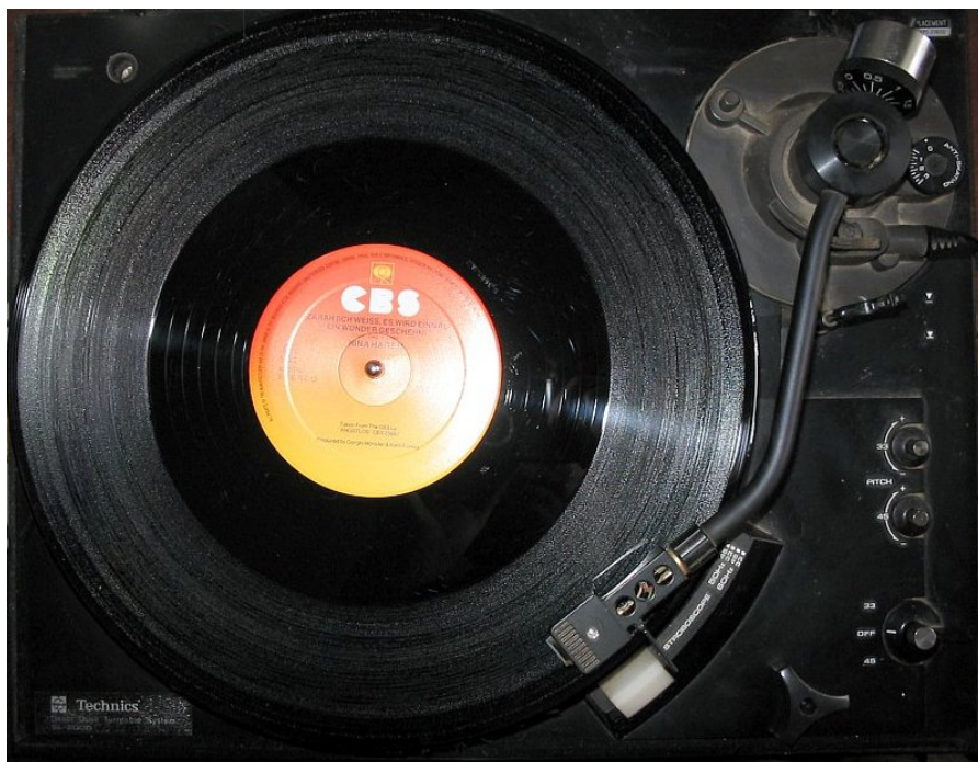
Figure 6: A turntable, or phonograph , is an electromechanical instrument. Source [56]
