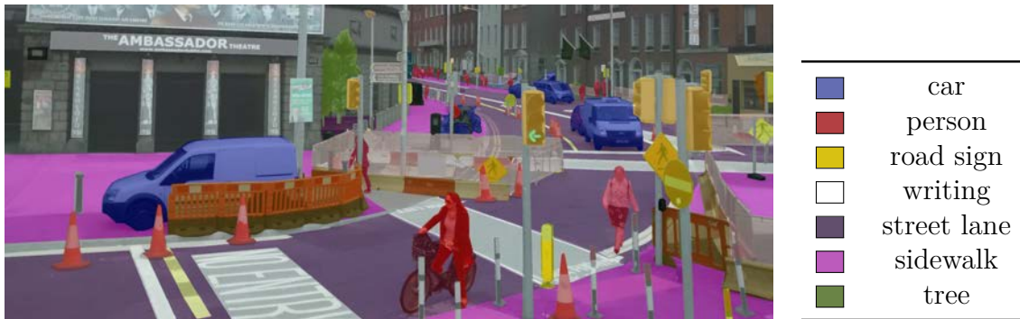
Figure 1.1: Semantic segmentation of a 2D image depicting an outdoor environment. Labels are represented by different colors superposed to the original image.
