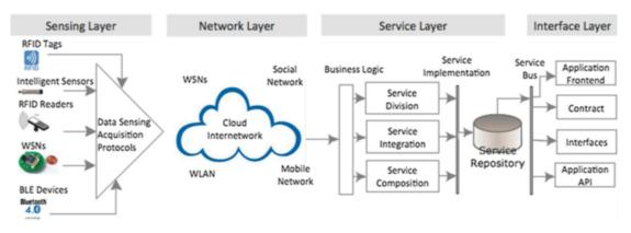
Figure 9 - Service-oriented architecture for IoT (Li et al., 2014)
