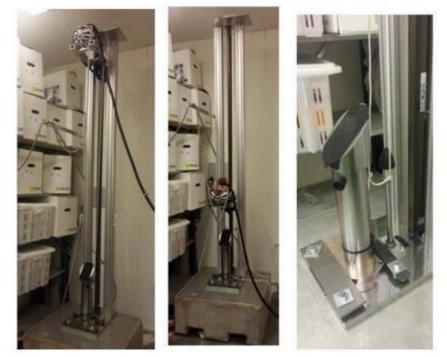
**Fig. 6:** The oblique test rig used to perform the three drop tests at the MIPS. The 45° angled steel anvil is shown on the right.
