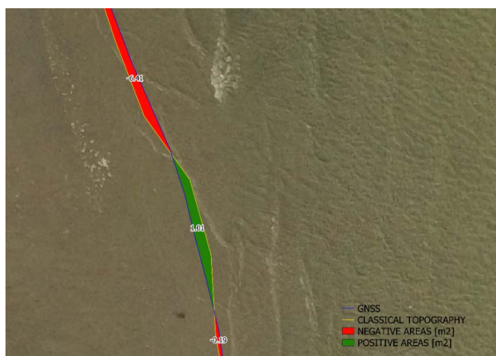
Figure 81 Layer union with positive and negative areas for calculating mean and standard deviation.
