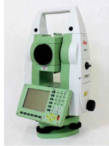
Figure 9 Total Station for measuring angles and distances (source: faradsrl.it).
