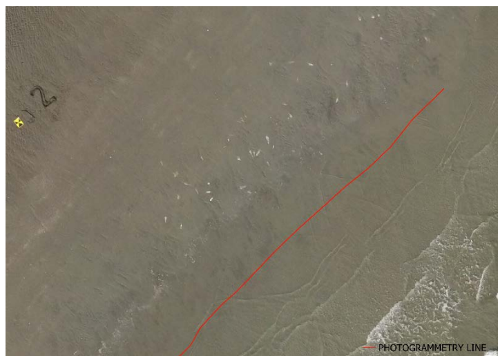
Figure 82 Plotting the coastline from the orthophoto.
