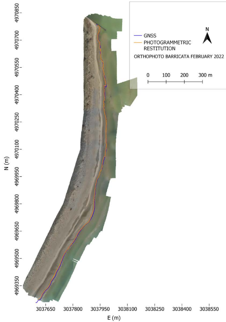
Figure 107 General framing coastline restitution lines (GNSS and photogrammetric restitution).
