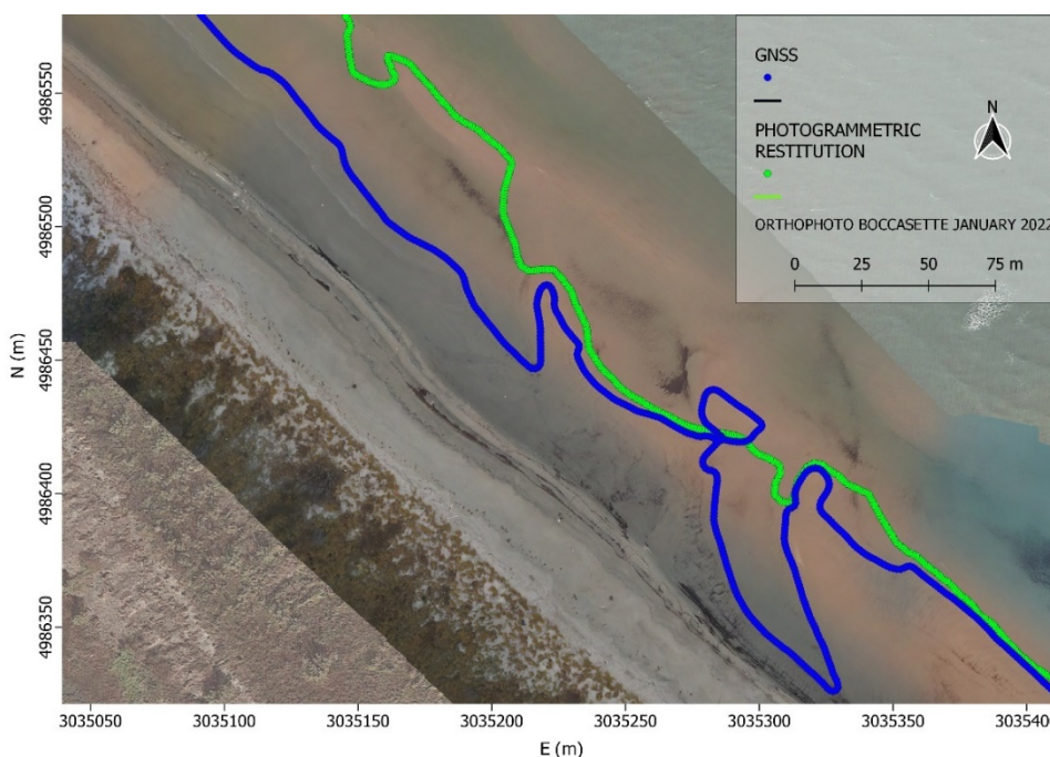
Figure 94 Very low correspondence between GNSS and photogrammetry.
