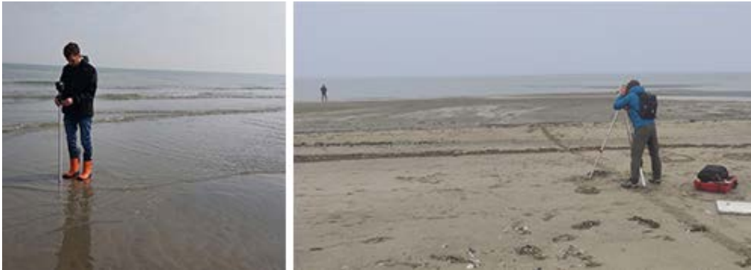
Figure 47 Measurement acquisition with Total Station in Boccasette.
