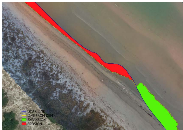
Figure 87 Local expansion and erosion, zero line in the Boccasette multitemporal comparison.
