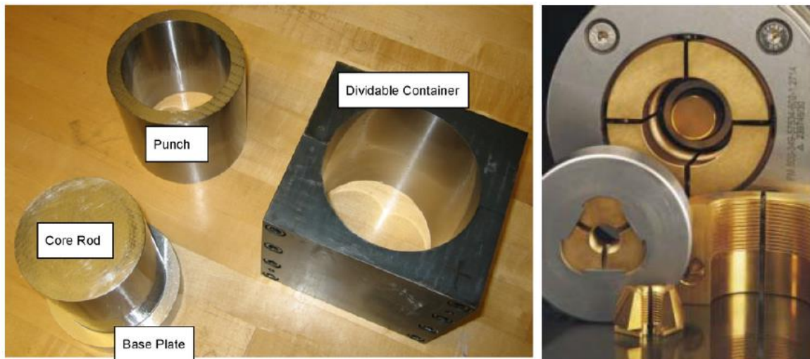
Figure 4.12: (a) Experimental set for split die (Chen et al. 2007), (b) thread forming die (Andersen & Lund 2008).
