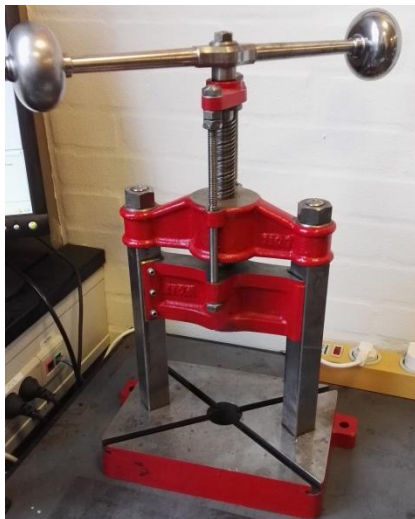
Figure 6.1: Mechanical press used in the experiments for powder compaction.
