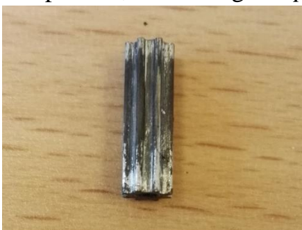
Figure 6.17: Detail of the residual aluminium stuck on upper punch.
