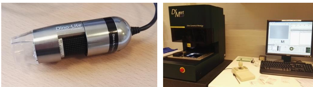
Figure 6.6: The two microscopes used in this project: the digital one on the left, the optical one on the right.
