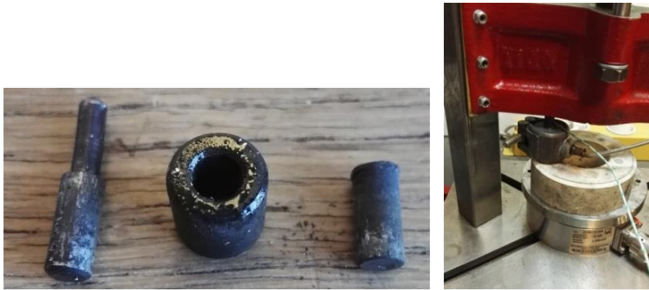
Figure 6.5: On the left, the cylindrical die-set used in these experiments; on the right, a phase of the sintering process.
