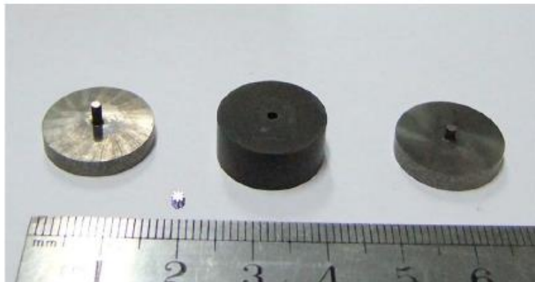
Figure 3.6: Die-system, respectively upper and lower punches, die and generated micro-gear (Dong Lu et al. 2013).
