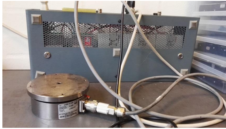
Figure 6.3: Plate and system used for the force measurements.
