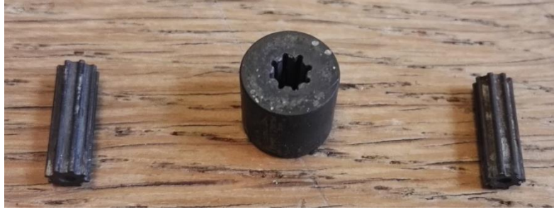
Figure 6.8: Die-set for the experimental gears. From left to right, upper punch, die, and lower punch.
