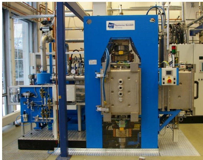
Figure 2.24: SPS work station. Note. From: www.ifam.fraunhofer.de .
