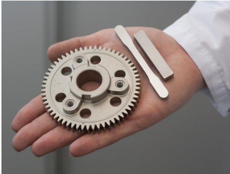
Figure 2.26: Geometry complex sintered parts. Note. From: www.tuwien.ac.at .
