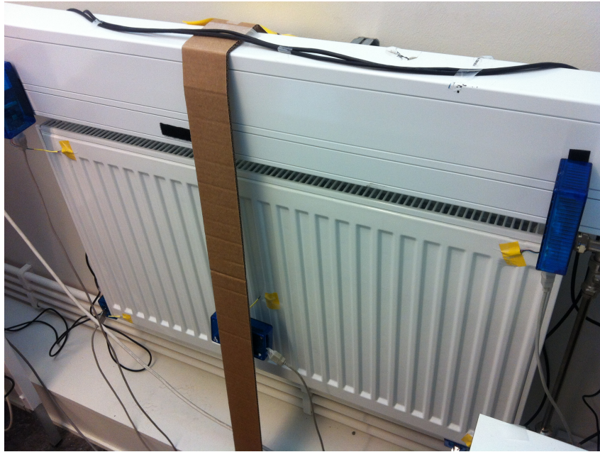
Figure 3.7: Picture of the notes attached to the radiator to run the test to get the mean radiant temperature.
