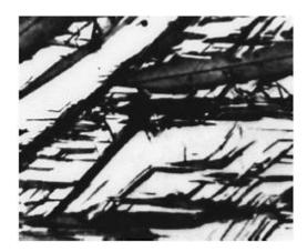
**Fig. 1.15** Retained austenite (white) trapped between martensite needles (black) (x 1000).
