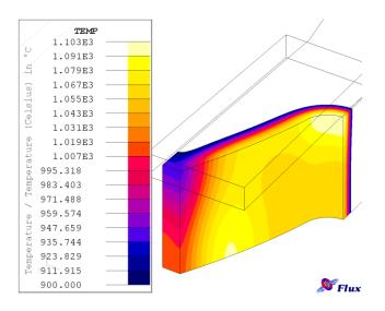
Fig. 4.10 900°C isotherm at the end of HF heating, recipe D
