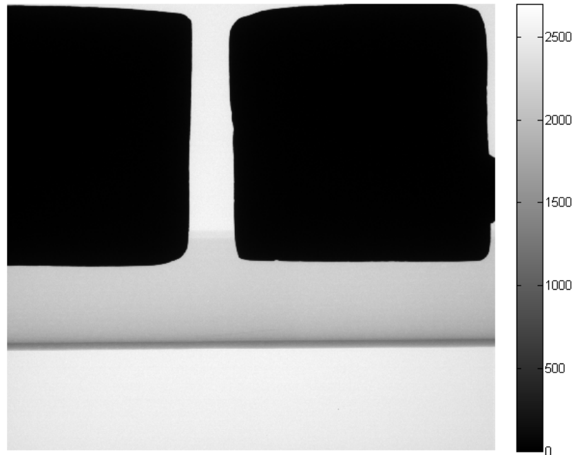
Figure 3.20: Acquired image of the detector's panel with two lead plates in front of it (50th frame, 45 kV, 800 \mu A, 500 ms p.w., 1000 ms f.t.).
