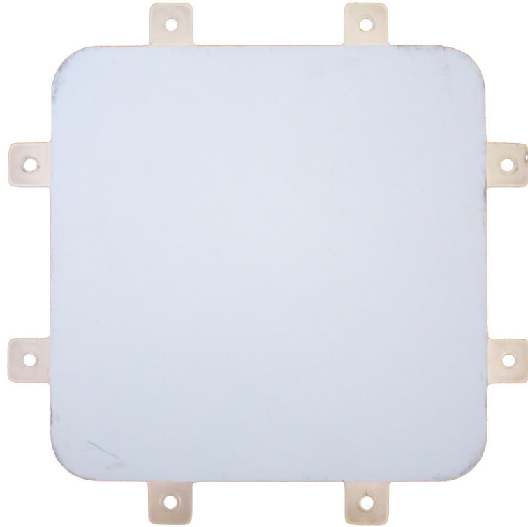
Figure 3.6: The internal plate with its light blue thermal pad attached
