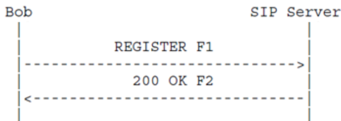
Figure 7: unauthenticated call-flow for a REGISTER request.
