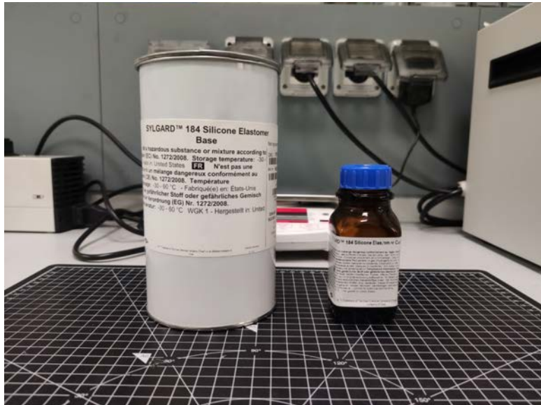
Figure 3.11 PDMS Sylgard® 184 (Dow Corning), two-part kit: silicone elastomer base on the left, curing agent on the right.
