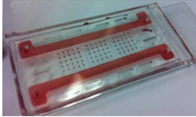
Figure 1.1 Example of a microfluidic device. A microbioreactor composed of a matrix of microwells arranged in lines and connector to two lateral channels. The Device is filled with a color tracer that allows the visualization of the structure. Adapted from 3 .
