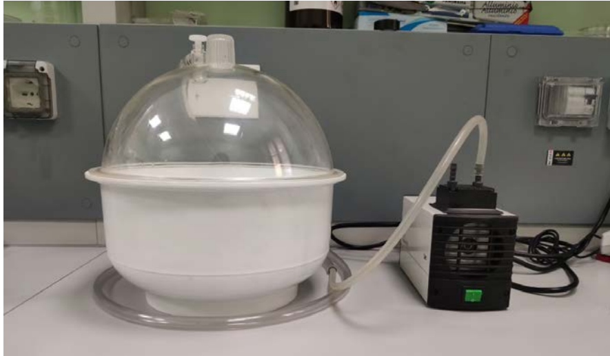
Figure 3.14 Desiccator connected to a vacuum pump in the BIAMET laboratory.
