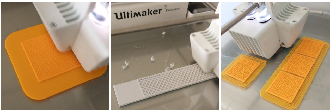
Figure 1.6 From left to right, infill pattern: grid, octet, cross 3D
