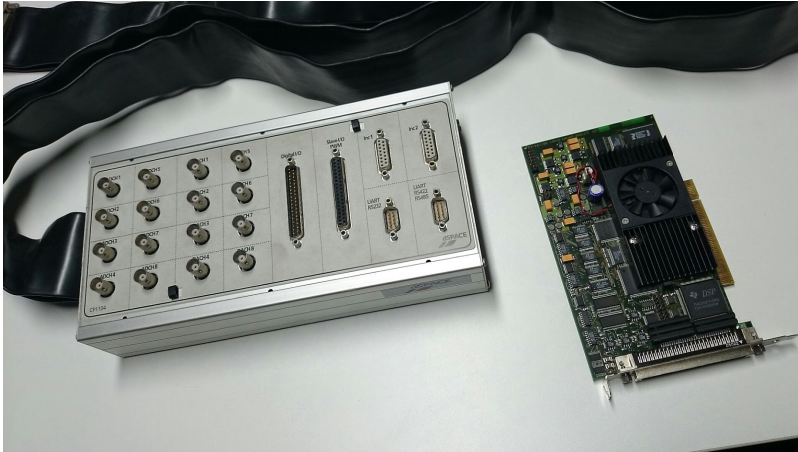
Figure 2.17: DS1104 PCI board and CP1104 connector panel.
