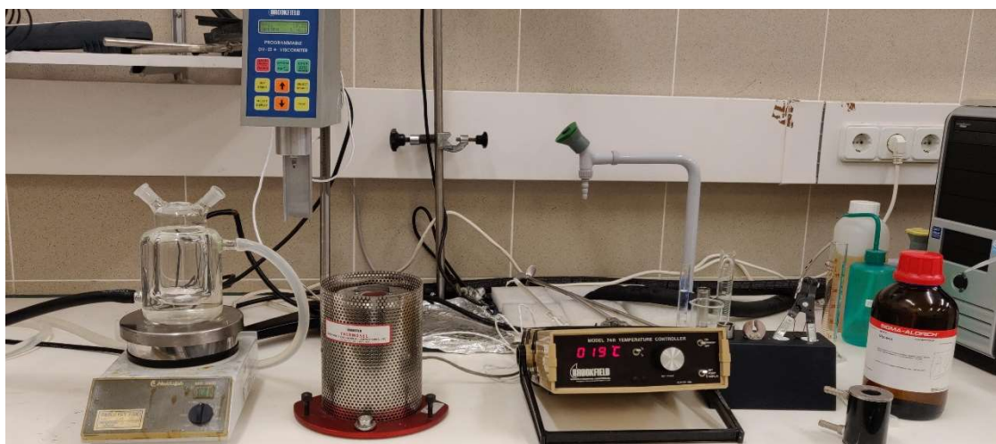
Figure 2.5. Thermosel, Viscometer and reactor used to calculate the calibration curves.
