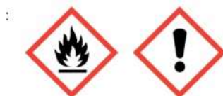
Figure A.3. Pictograms of the dangers regarding the handling of Sodium Methoxide
