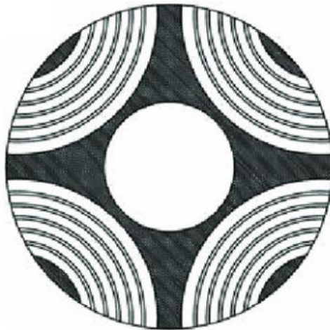
Fig 2.2: Multiple barrier rotor design
