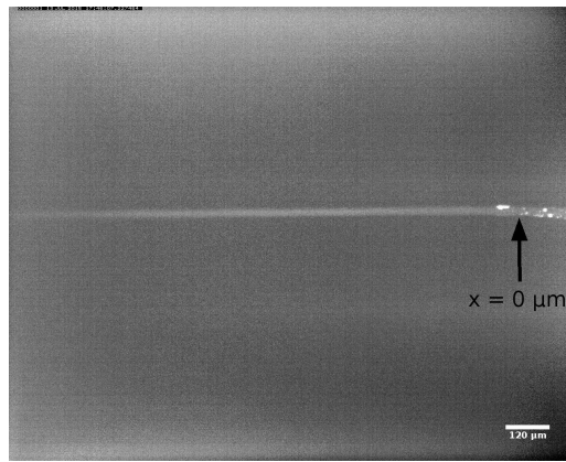
Figure 3.24: Origin point for the x -axis. Picture taken with a 6 mm high sample solution column and a 2000 \mu\text{L}/\text{h} sheath flow rate.
