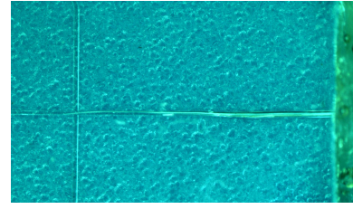
(b) The capillary can also bend when inserted into the PDMS channel.
