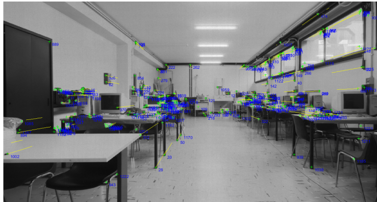
Figure 5.2: Glimpse of the viewpoint of the left camera. The blue crosses are detected features and yellow lines are the associated features motion
