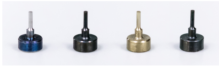
Figure 22. Cores: the first from the left is uncoated, the second is coated with DLC-1, the third is coated with CrTiNbN, and the fourth is coated with DLC-2.
