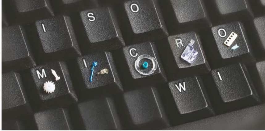
Figure 2. Examples of micro devices produced by injection moulding.
