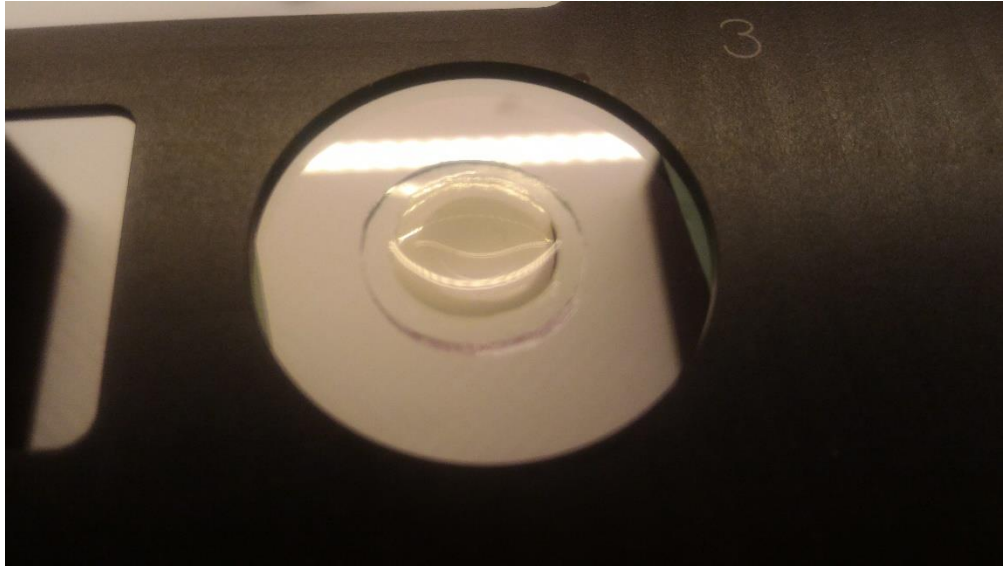
Figure 4.8 Upper side of the sample for evonik silicone fabrication. Liquid silicone is contained by a PDMS gasket placed on the glass substrate
