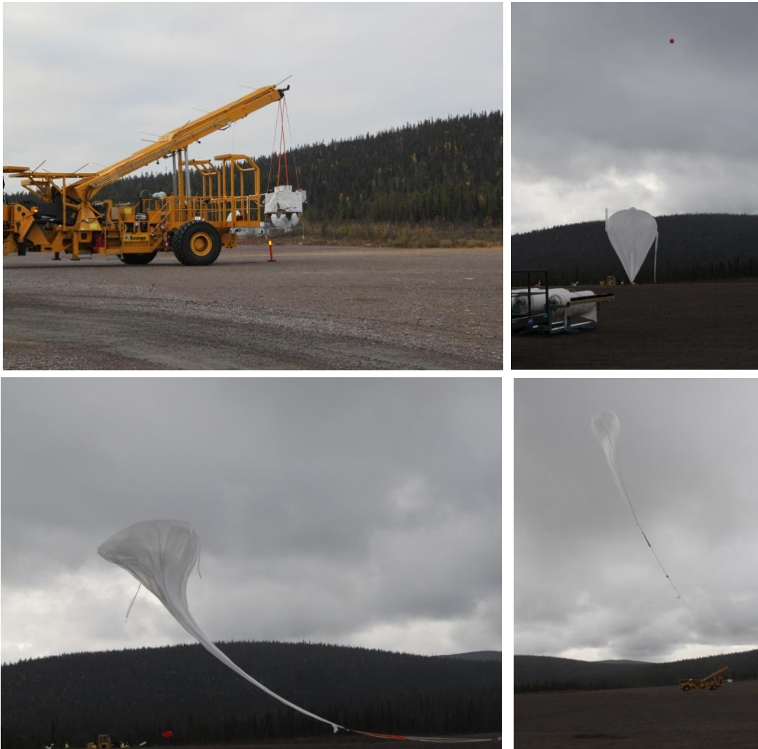
Figure 35 The Hercules vehicle transports BX15 on the launch pad, balloon inflation and release sequence before launch on 25th September 2012
