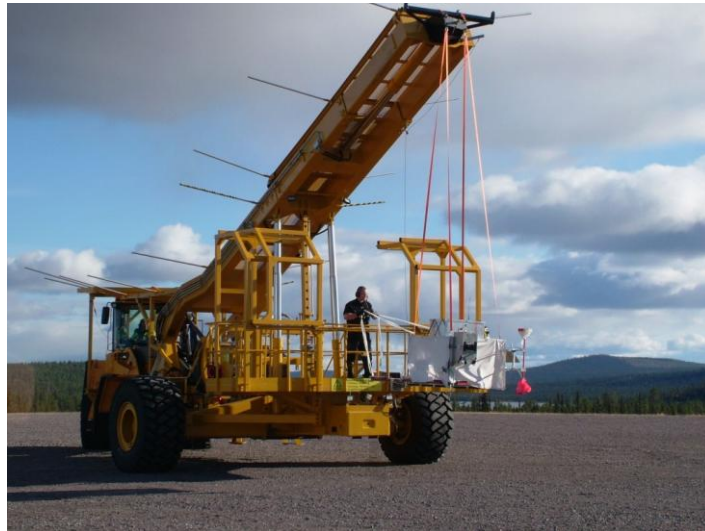
Figure 33 Pick-up of the BX15 gondola by Hercules before the FCT, from this picture MISSUS onboard was placed on the left side
