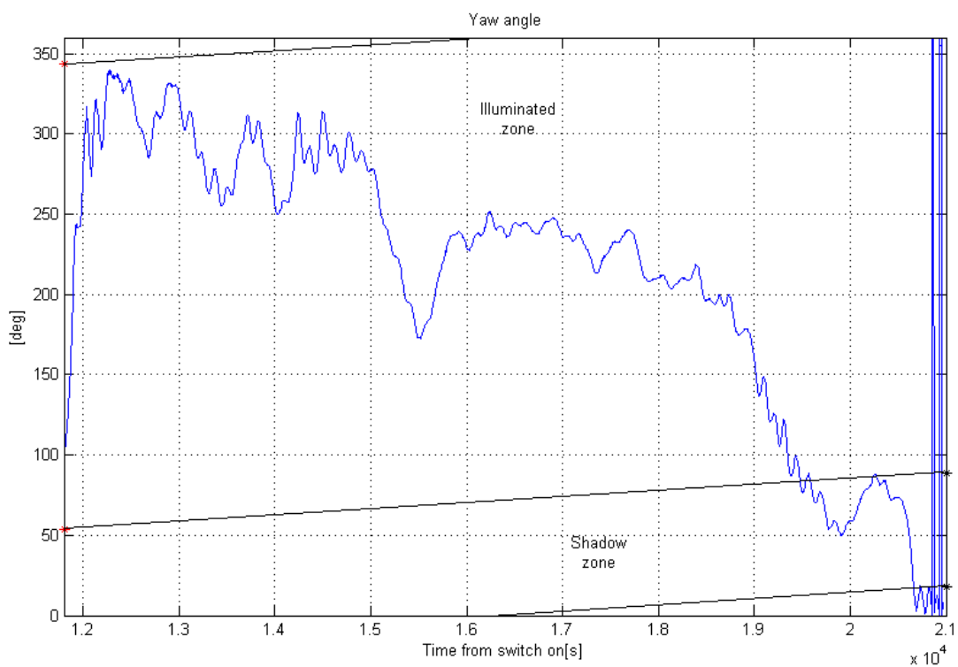
Figure 93 Yaw rotation during cruise and variation of the shadow zone
