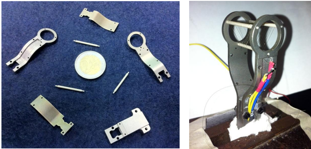
Figure 14 Sensor's components compared with a euro coin (left), assembling of the RTD Sensor (right)
