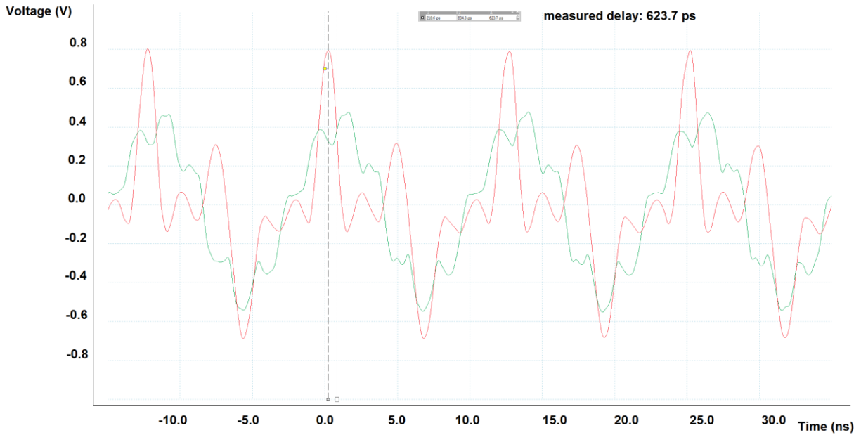
Figure 4.9 Measurement of the delay between pump (red) and external trigger (green) signals at the oscilloscope
