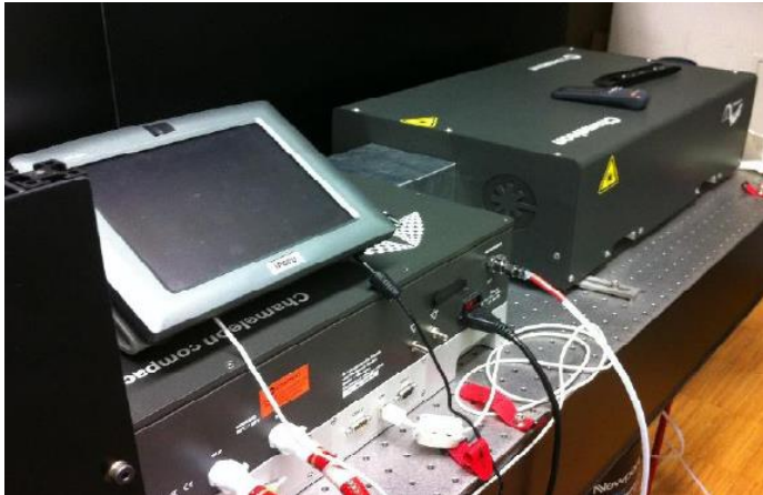
Figure 2.3 Laser sources: OPO on the left, pump on the right
