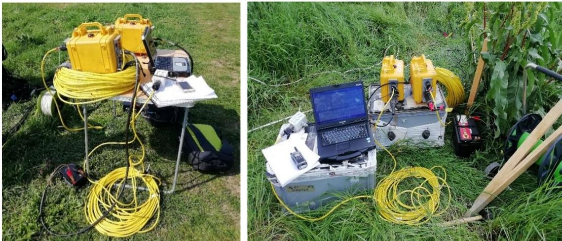
Fig. 3. 12, Geode Exploration seismographs from the University of Padova, used during the field work
