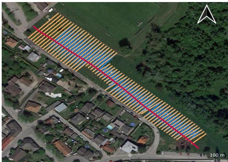
*Fig. 5. 14, Distribution of measurement points from the CMD-Explorer: the area mapped (direct -orange- and diagonal -blue- lines) and the longitudinal -red- profile, georeferenced and plotted in QGis*
