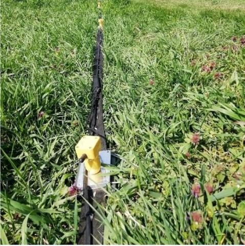
Fig. 3. 16, Geophones on land streamer, adopted for the first acquisition
