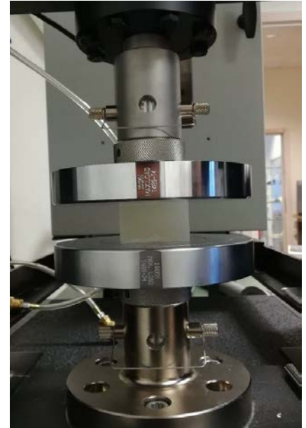
Figure 5.8 - Silicon Rubber sample compression test
