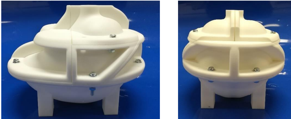
Figure 4.8 - 3D printed mould designed for Brain casting and sensors positioning of IHHS 2.0
