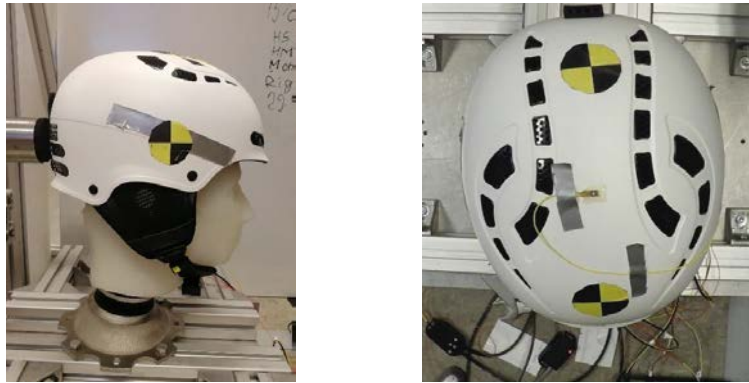
Figure 4.34 - Accelerometer applied externally on the apex of the Helmet.
