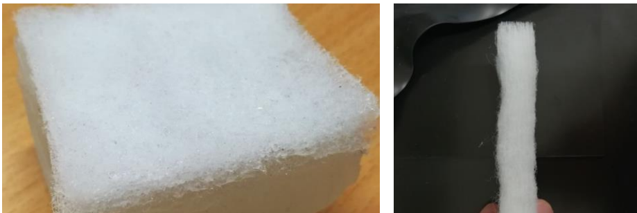
Figure 5.12 - Nonwoven Fabric used as Arachnoid substitute in the Dummy Head prototype a) Non-woven fabric coupled with silicone rubber b) Non-Woven Fabric testing sample thickness
