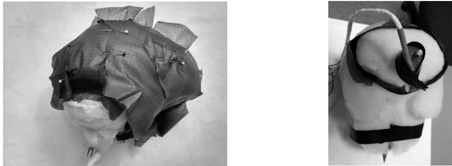
Figure 3.5 Wrapping of the brain with nylon sheet to mimic the SAS
