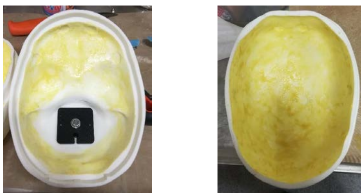
Figure 4.14 - Dura Mater substitute in IHHS 2.0; thin layer of silicon glue is spread over the inner surface a) bottom skull part b) top skull part
