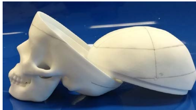
Figure 4.4 - Side view of IHHS2 3D polyamide printed parts with FORMIGA P110
