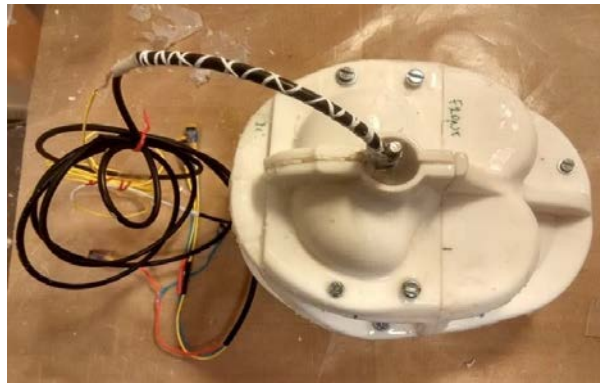
Figure 4.12 - Brain casting procedure: a) The threaded stem is put in the rubber and cured together with the lower part b) Closure of the brain mould and curing time
