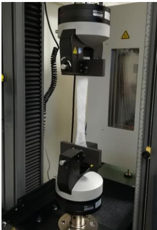
Figure 5.14 - Non Woven Fabric tension test a) Setup of the sample on Instron traction Machine b) Nonwoven Stress vs Strain tension test
