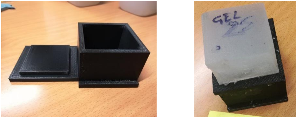
Figure 5.7 - Specimen Mould preparation, rubber sample demoulding and test setup
