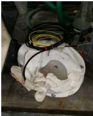
Figure 4.12 - Brain casting procedure: a) The threaded stem is put in the rubber and cured together with the lower part b) Closure of the brain mould and curing time
