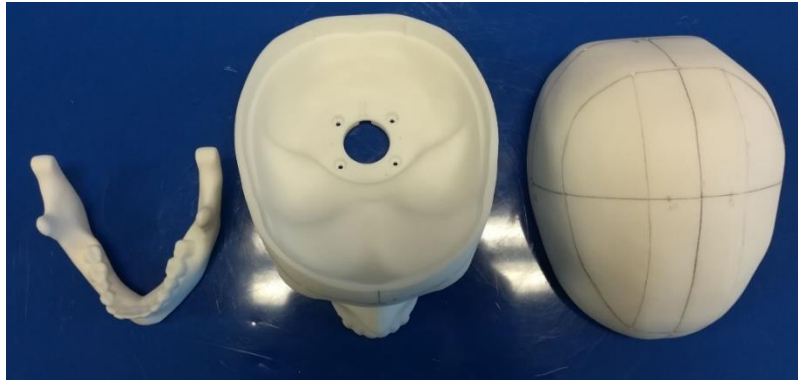
Figure 4.3- Top view of IHHS2 3D polyamide printed parts with FORMIGA P110
