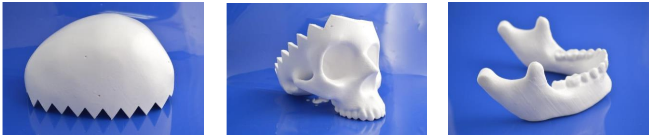
Figure 3.2 IHHS 1.0 3D Printed Skull a) Top Part b) Bottom Part c) Jaw
