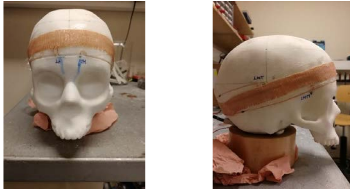
Figure 4.20 - The connection between the upper part and the lower part of the skull are connected using the silicon Rubber glue
