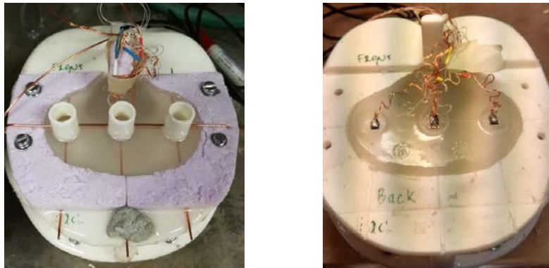
Figure 4.11- Brain casting procedure: a) Cerebellum casting with cylinders for sensors spots localization b) Embedding of sensors in the correspondent position of cerebellum
