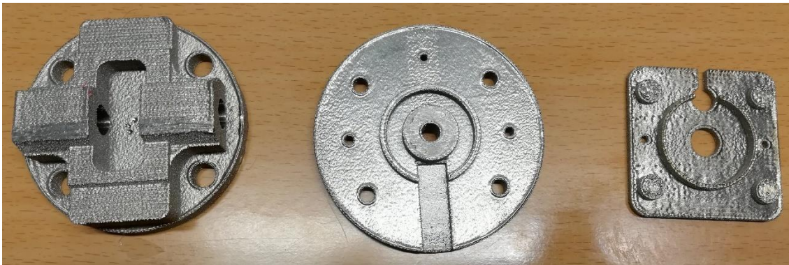
Figure 4.30 - Customized Neck Adaptor parts printed with EBM machine. Left) Skull-Neck Adaptor; centre) External part; right) inner part
