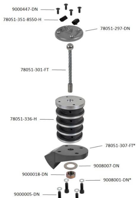
Figure 4.31 Neck Assembly Hybrid III 50th-percentile
