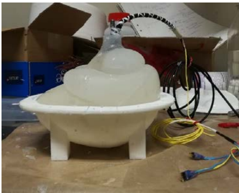
Figure 4.13 - Brain casting procedure: Brain demoulding and particular of the complete rubber component with the connection wires
