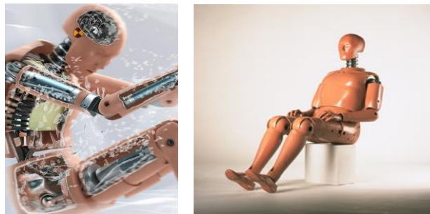
Figure 1.1 - Anthropometric Testing Device "Human Hybrid III"
