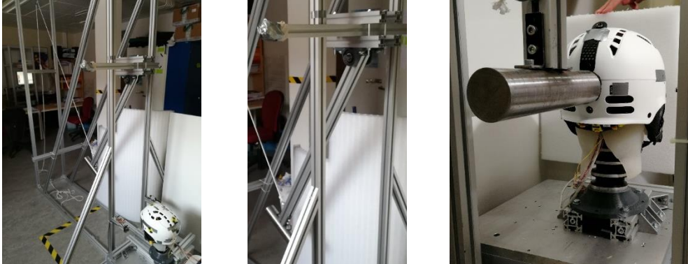
Figure 3.15 Impact Frame structure and impact point
