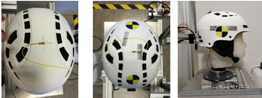
Figure 3.25 - Helmet configuration with the apex accelerometer glued on the top part, this sensor will collect the energy reached directly from the pendulum
