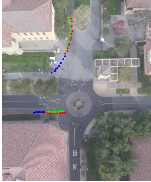
Figure 1.1: Example of trajectories on deathcircle scene of SDD dataset Blue: observed agent positions. Red: predicted future agent positions. Green: real future agent positions.
