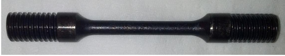
Fig 4.4b Samples of Thin-Walled Tubular Specimens used for the Tests in Tekniker.
