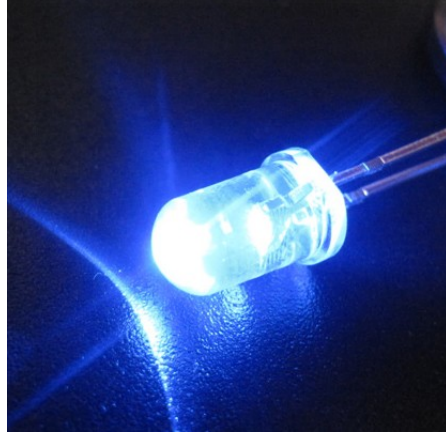
Figure 5.4: The LED source of operative wavelength \lambda = 470 \text{ nm} .
