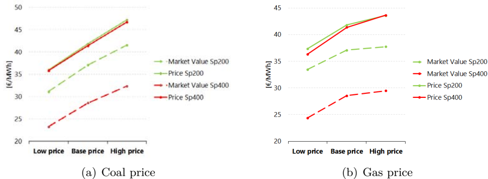
Figure 10.13: Change in wholesale electricity price and MV for difference levels of coal and gas prices.
