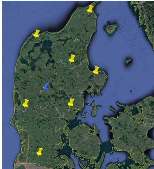
Figure 8.7: Locations from which wind speed time series are extracted. In blue, the reference location (Herning) is shown.
