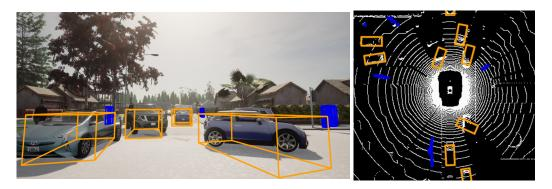
Figure 5.4: Front view (left) and BEV (right) of predicted bounding boxes of camera-only model.
