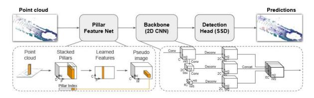
Figure 3.3: Pointpillars network structure [12].
