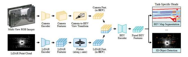
Figure 3.5: BEVFusion network structure [14].
