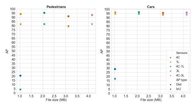
Figure 5.3: AP for multiple sensors object detection. Pedestrians AP in the left and car AP in the right.
