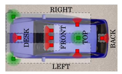
Figure 3.1: Sensors positioning on the simulation car. Green sensors are LiDARs and red ones are cameras.
