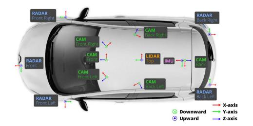
Figure 4.9: Sensor positioning on the nuScenes car.
