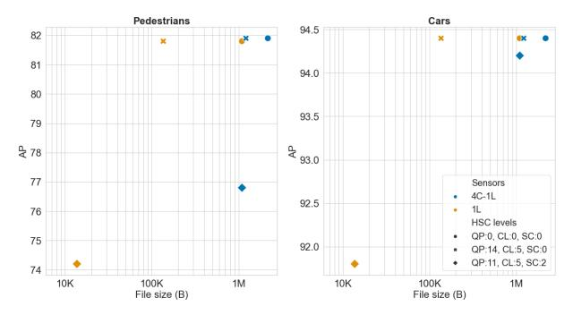
Figure 5.6: AP results for LiDAR-only and BEVFsuon models using compressed point clouds. Pedestrians AP in the left and car AP in the right
