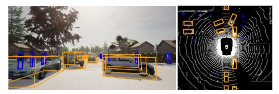
Figure 5.5: Front view (left) and BEV (right) of predicted bounding boxes of LiDAR-only model.
