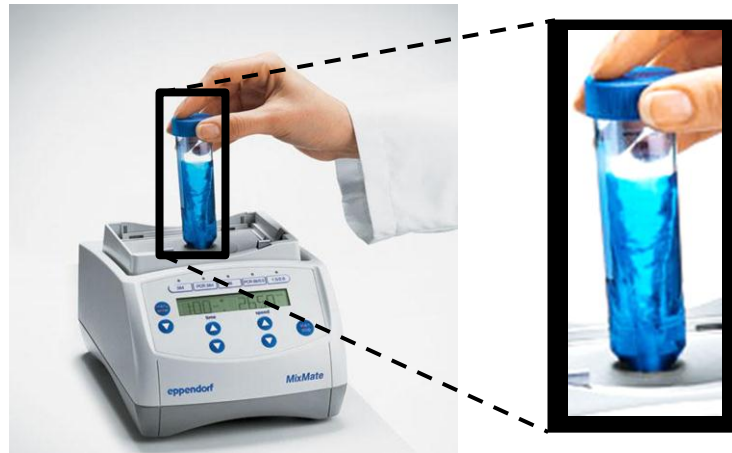
Fig 1.4: Vortex mixer (left) and the induced vortex (right) Picture taken from http://www.pocdsscientific.com.au .
