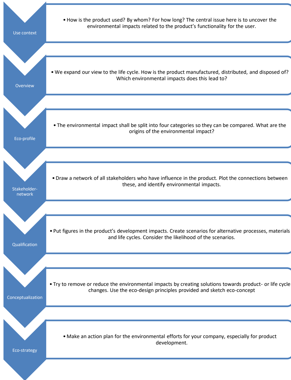
Figure 7 – 7 Steps towards environmental improvement. (McAloone & Bey, Environmental improvement through product development. A guide , 2009)
