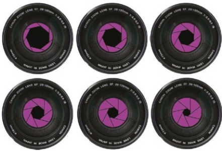
Figure 4.3 Top row (left to right): f/4, f/5.6, f/8; bottom row: f/11, f/16, f/22.
