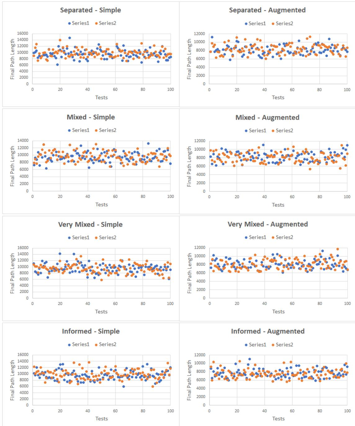
Fig. D.1: *Environment 1: Uniform Rotational Sampling*. The final path length of the path after the smoothing of the first (light blue) and second solution (orange), on the left with the Simple RRT, on the right the Augmented.
