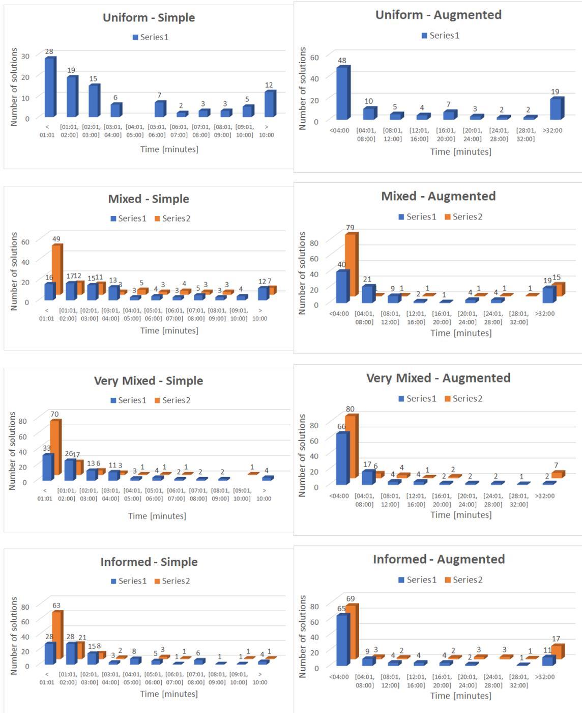
Fig. 3.13: Time required for the computation of the first (light blue) and second solution (orange) with all sampling techniques on both the algorithms (Simple RRT on the left, Augmented RRT on the right).
