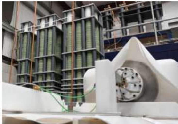
Fig 2.8: The pneumatically-controlled spark gap and variable resistor array
