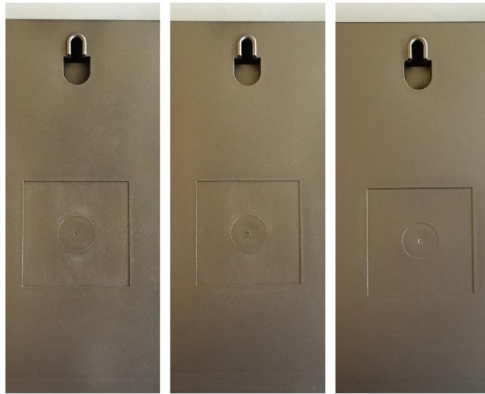
Figure 3.21 Verification of the differences in painting using different instruments: in the images of the left and center was used the airbrush, in the right one we used a spray gun.
