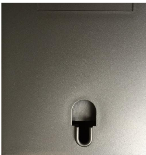
Figure 3.11 Surface irregularities caused by agglomerates of CNTs (Sol 1,2 ): irregularities are identified looking at the dark dots in the light gray background (bottom-right) and light dots in the dark gray background (top left).
