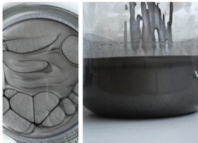
Figure 3.8 Sol 2.1 after 30 minutes of mixing with the magnetic stirrer.
