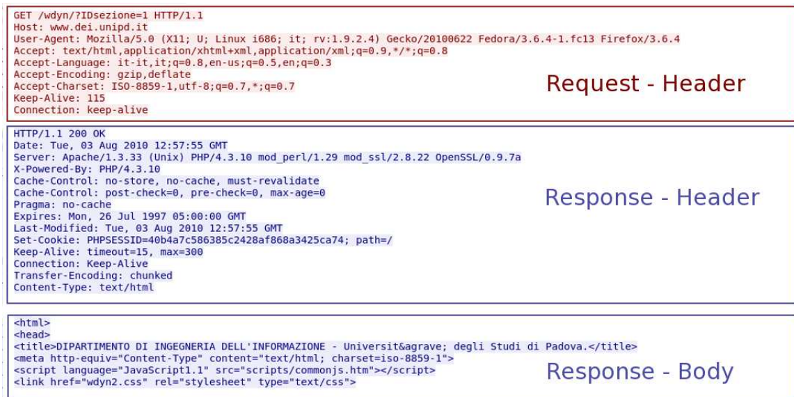
Figure 2.25: HTTP session with GET method examined using WireShark [19]
