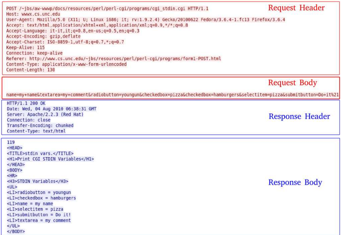
Figure 2.26: HTTP session with POST method examined using WireShark [19]
